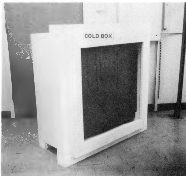
Figure 2. Separated View of Guarded Hot Box Apparatus
