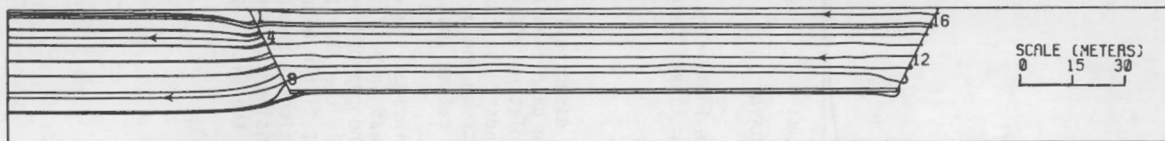
FIGURE 34. Pathlines of Tailings Leachate--Below the Water Table, with Bottom Liner, Case 6
