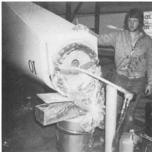
Figure 57. - Blade ballasting process.
