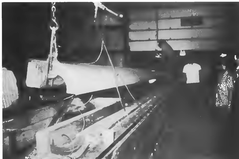
Figure 44. - Preparation for blade half-shell bonding.
