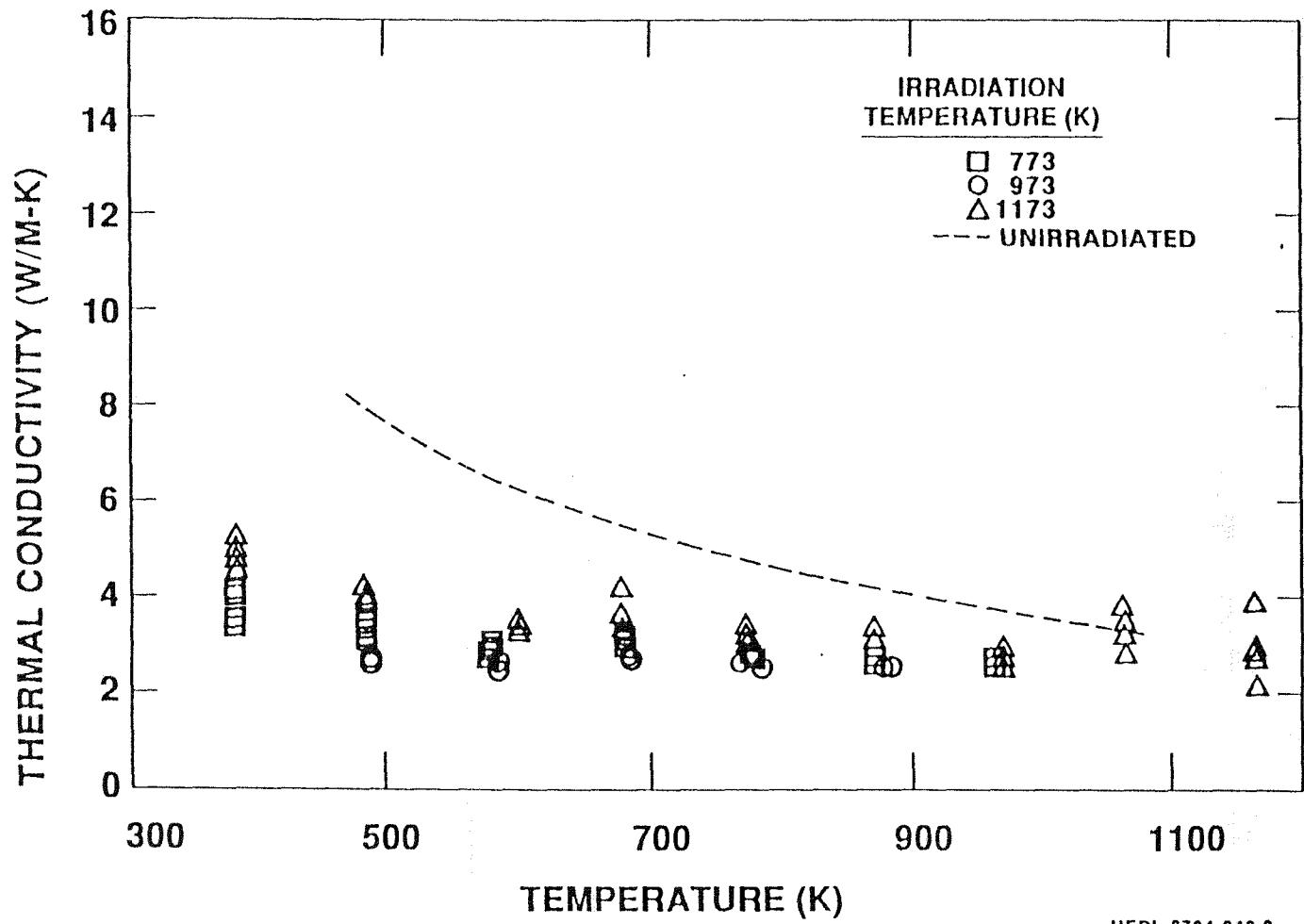
FIGURE 8: Thermal Conductivity of  $\text{LiAlO}_2$  at Different Irradiation Temperatures -
