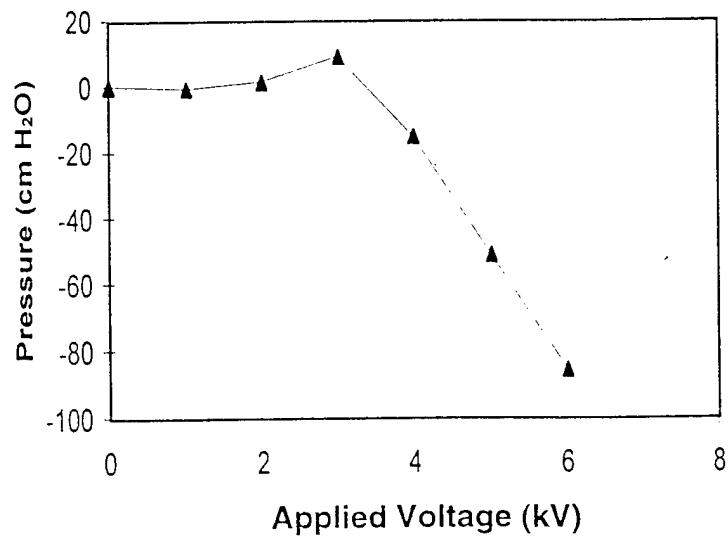
Pumping and Spraying of Air in Water
