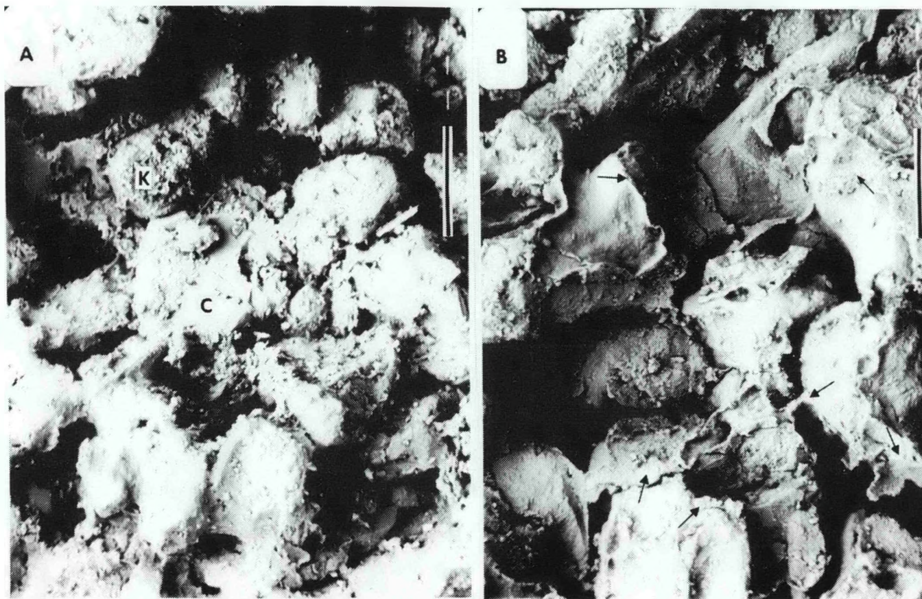
FIGURE 51. - Scanning electron micrographs of late stage cements. (A) Five percent calcite (C) cement in addition to 3 % clay (K) and 1 % siderite cement are the reason that permeability in this sample is less than 1 millidarcy. Well C-6, 4,422.6 ft (1,349 m). (B) Five- to thirty-micron thick clay cement (arrows) coats reduce an otherwise good reservoir sandstone to 236 md permeability. Sample from W-14, 4,297.7 ft (1,311 m). Scale bars are 100 microns long.
