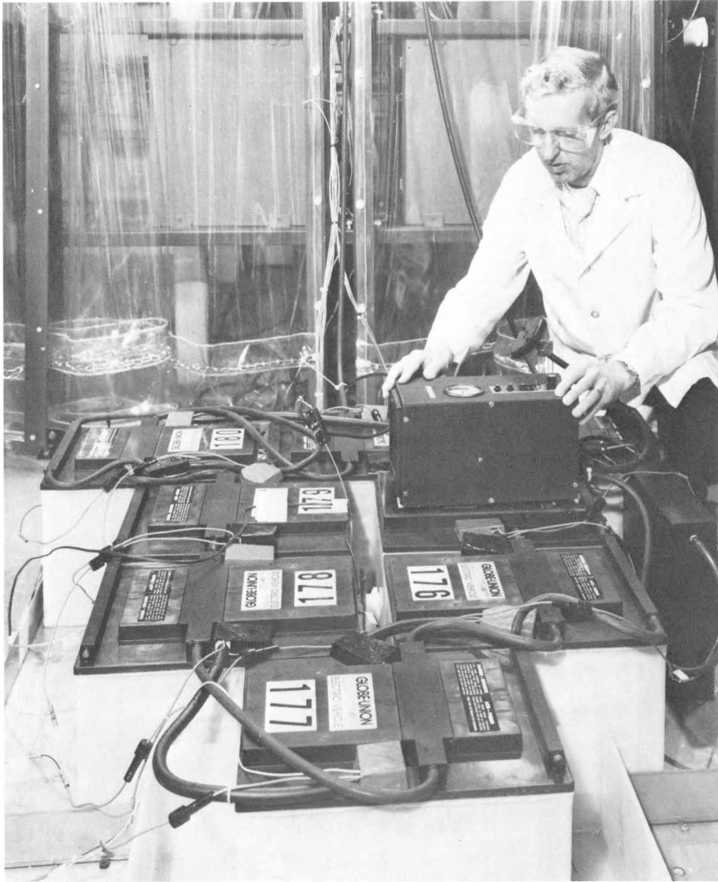
Figure III-1: A Globe 23.4 kWh, 96 V, Improved Lead-Acid Electric Vehicle Battery with Air-Induced Electrolyte Stirring System Under Test in the NBTL
