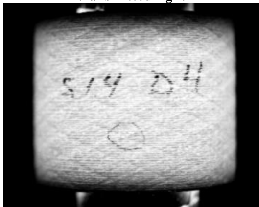
Figure 8: Hole in membrane visible in transmitted light
