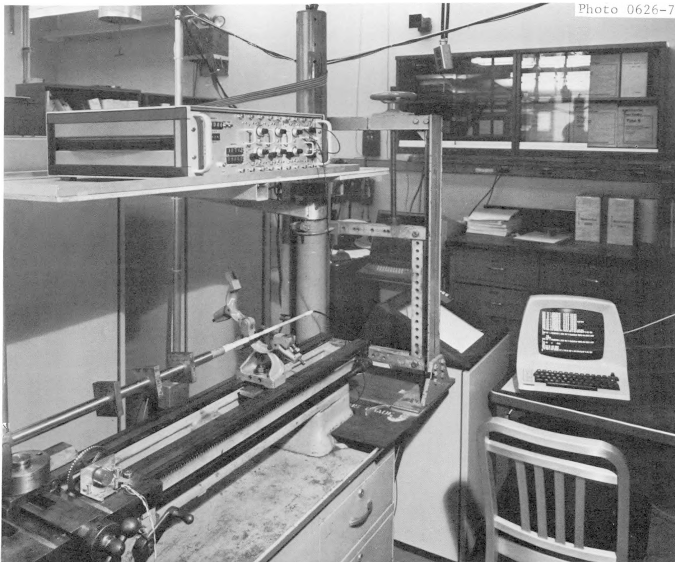
Fig. 10. Three-Frequency Eddy-Current Instrument, Tubing Test Bed, ModComp IV CRT Terminal, and Versatec Plotter.
