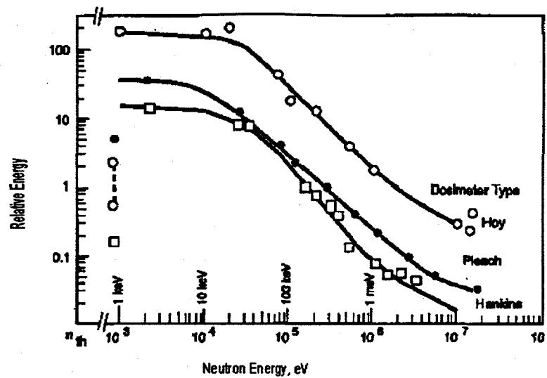
Figure 6.2. Energy Dependence of Various TLD-Albedo Dosimeters
