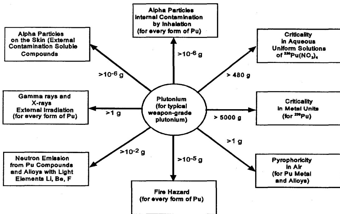
**Figure 2.4.** Hazards in Low-Exposure Plutonium Handling
