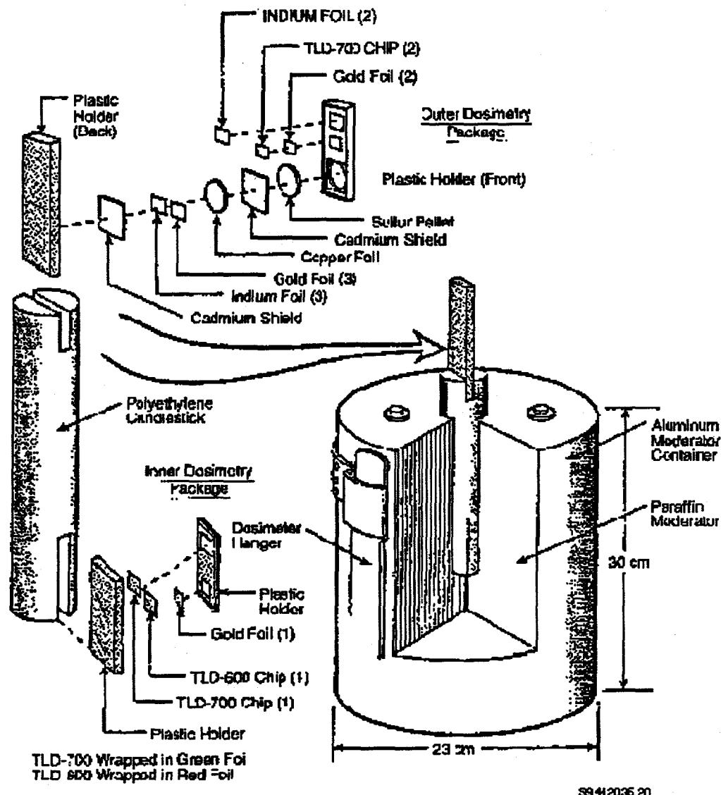
Figure 6.4 Fixed Nuclear Accident Dosimeter Used at Hanford to help Assess Doses from Criticality Accidents
