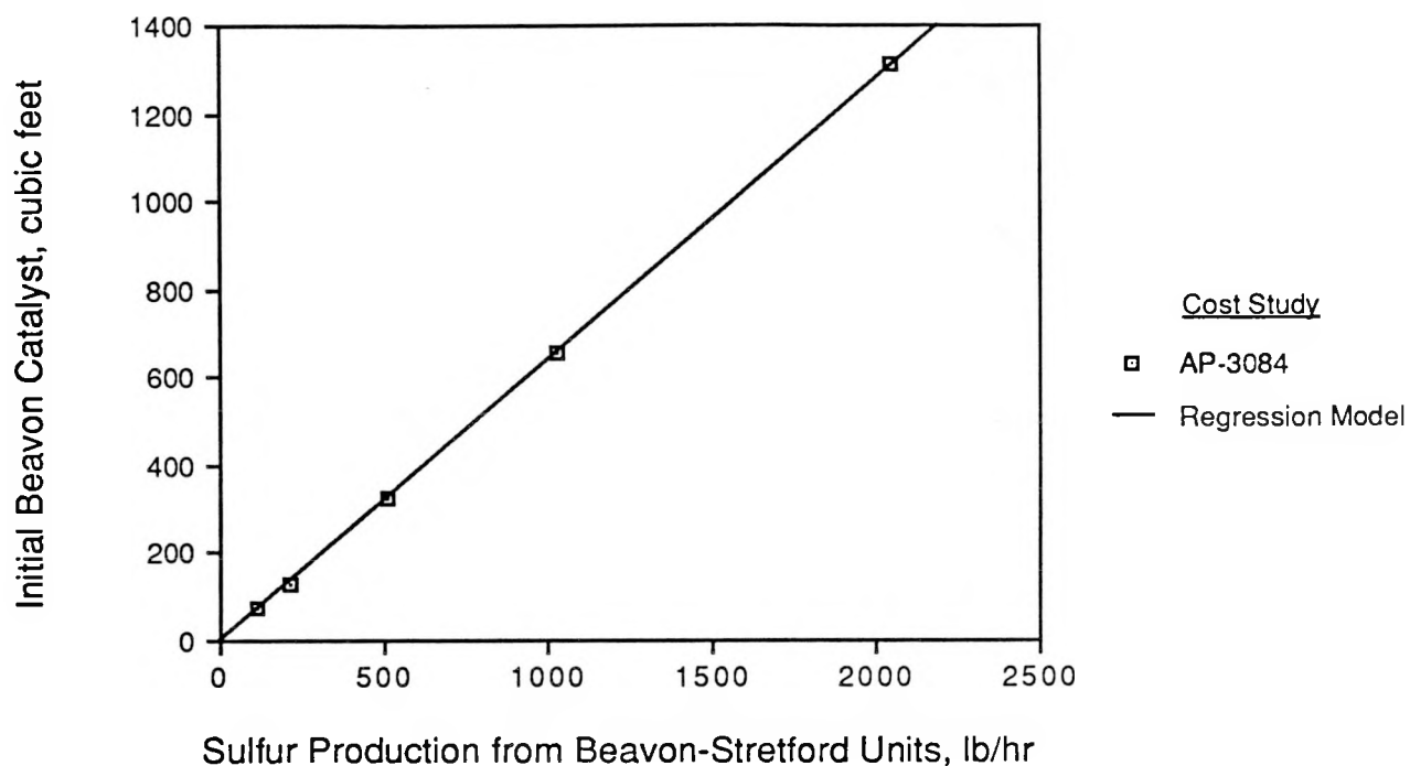
Figure 33. Initial Catalyst Requirement for the Beavon-Stretford Process
