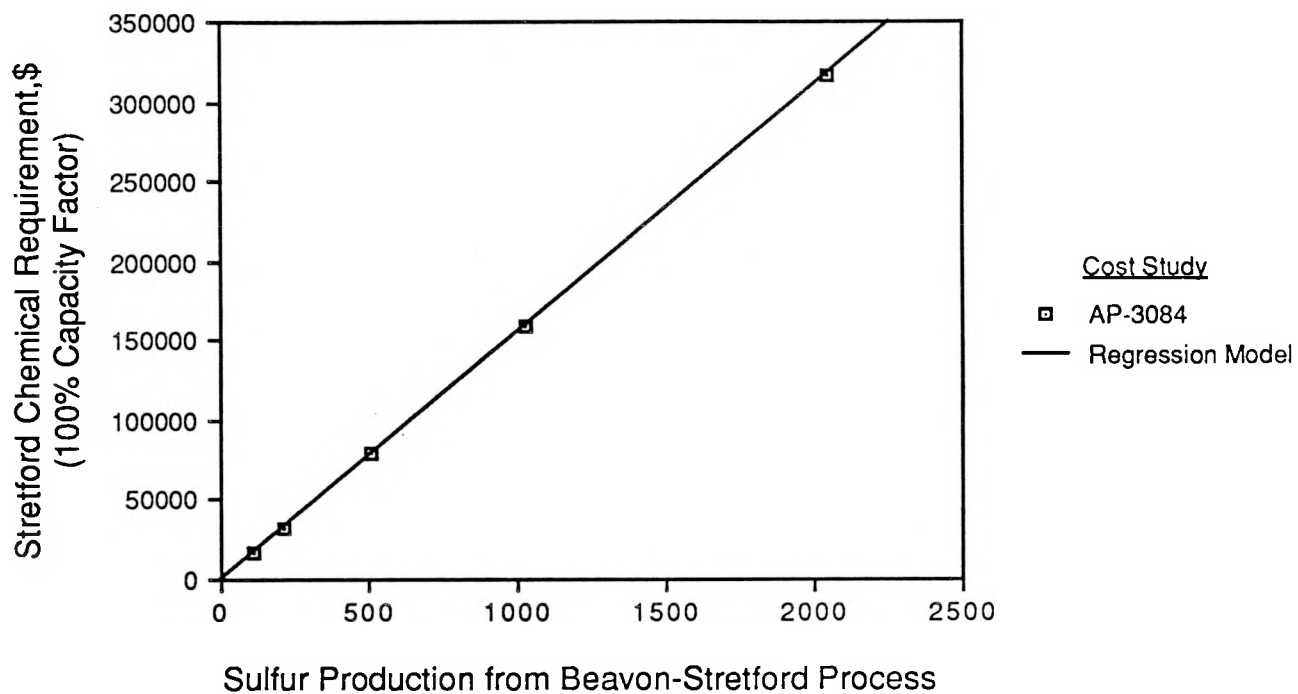
Figure 54. Annual Chemical Cost for the Beavon-Stretford Process
