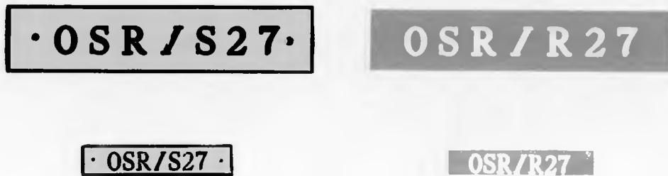
Fig. 2. Alternate labels used for instruments located in hostile environments are made of laminated plastic material to withstand all environmental hazards. (a) Yellow labels (large and small) with black lettering for Operational Safety Requirement safety system instruments. (b) Green labels (large and small) with white lettering for Operational Safety Requirement (limiting-condition) instruments.
