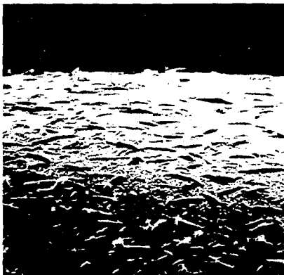
Fig. 26. SEM photograph showing typical surface growth caused by the reaction of alkali with water vapor and/or \text{CO}_2 in the air.
