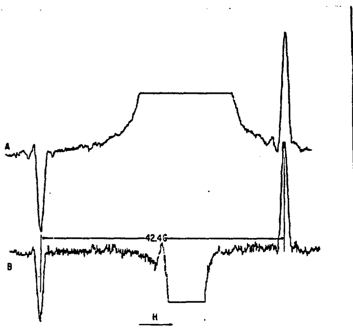
Figure 2. Field swept EPR spectrum of \cdot\text{CH}_2\text{CO}_2^- radical (pulse radiolysis) at 1 \mu\text{sec} after the electron beam pulse (B) central quartz signal reduced by beam-no beam subtraction.
