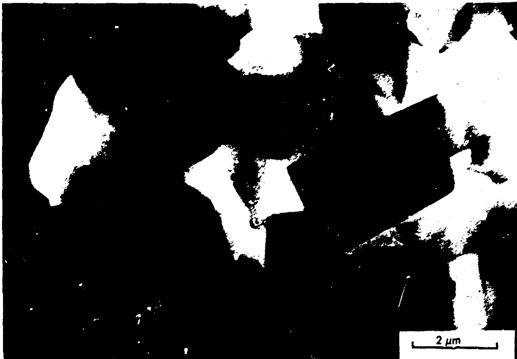
Fig. 4.15. Coors AD-85 alumina as received. (a) Optical micrograph showing \text{Al}_2\text{O}_3 grains surrounded by darker glassy phase. (b) Transmission electron micrograph.
