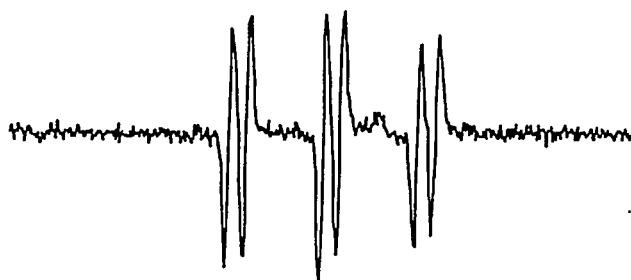
Figure 2. EPR spectrum (100 gauss width) of spin-adduct formed by discharge of a solution of 10 vol% methanol in water containing 0.01 M pyridyl- N -oxide- t -butylnitron.
