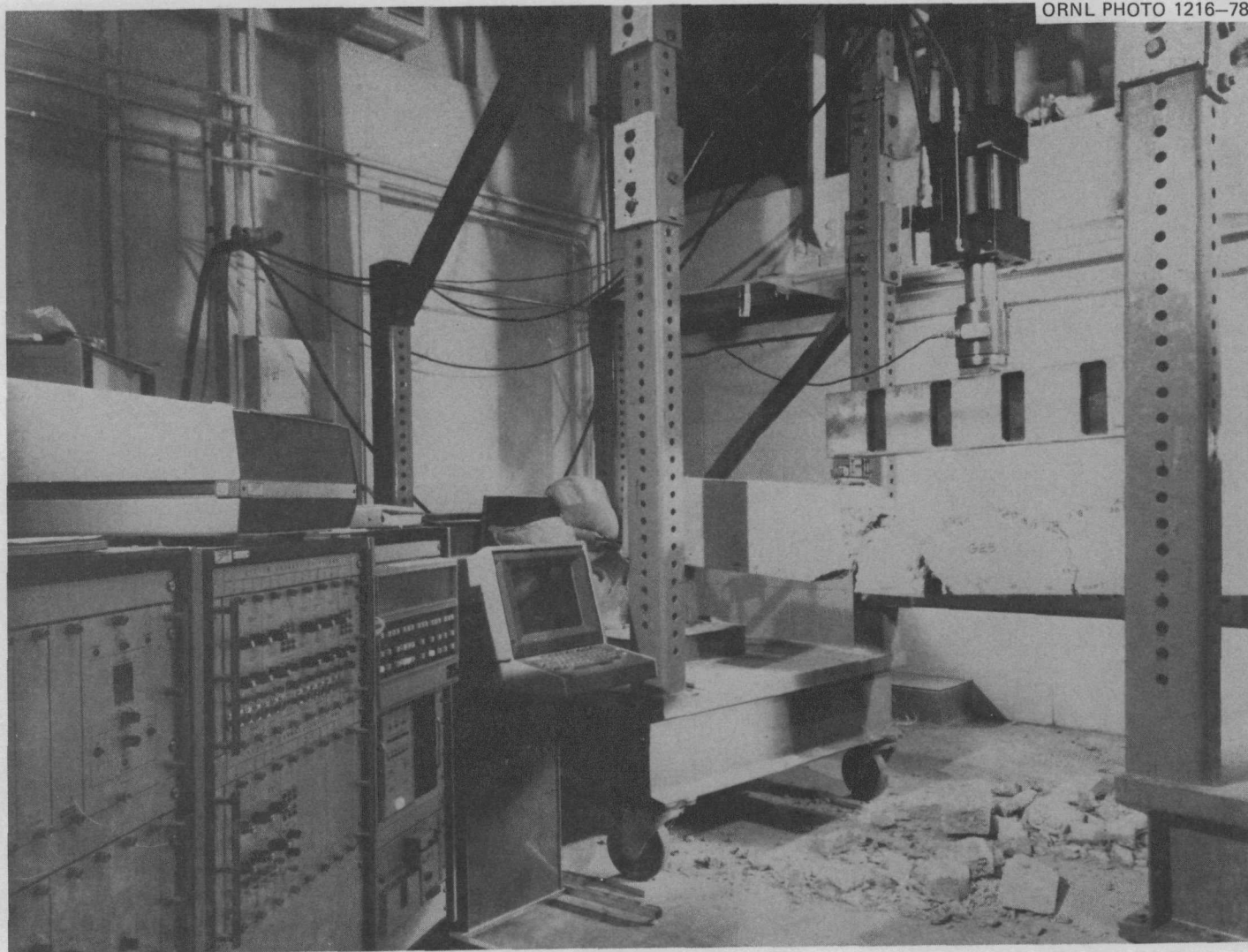
Fig. 104. Test setup for acoustic emission monitoring of posttensioned concrete beams.
