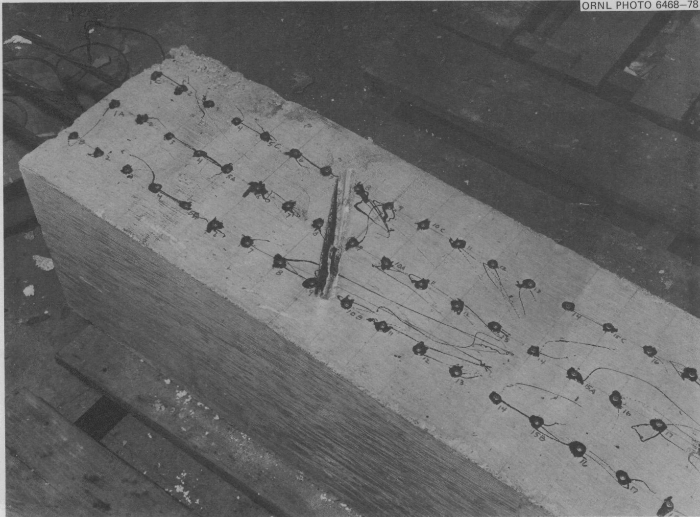
Fig. 30. Simulated failed tendon test specimen.
