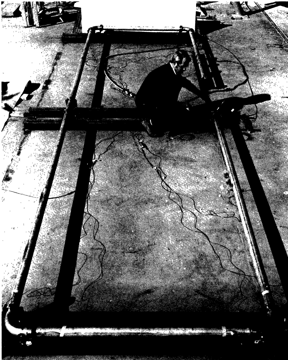
FIGURE 5 PIPING SYSTEM FOR THE OPEN RECTANGULAR LOOP EXPERIMENTS
