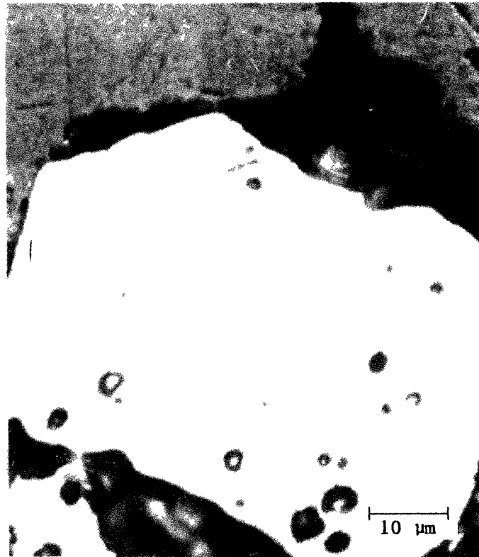
FIGURE 8. Granules Sintered in He/4% H 2 Fabricated and Sintered at SRL. Note Optimum Density that Results When Granules are Sintered in an Atmosphere that Reduces and Dissolves in Plutonia.
