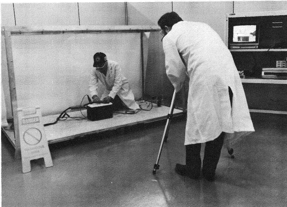
Figure 15. Ignition Testing of NI/FE Battery at INEL
