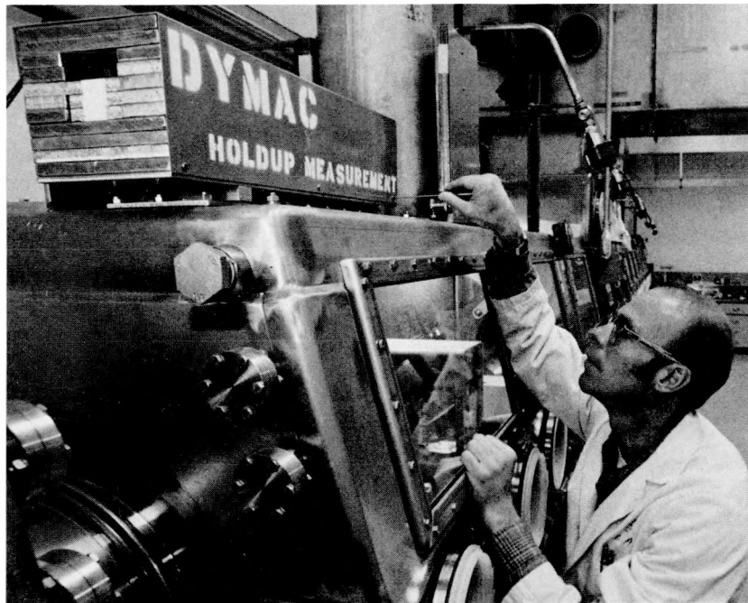
Fig. 66. Filter holdup monitoring system being installed on top of a glovebox.
