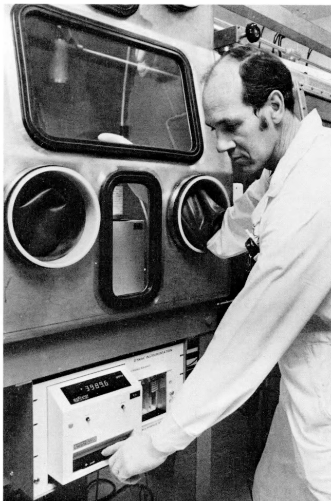
Fig. 57. Operator weighs a can of material on an electronic balance.
