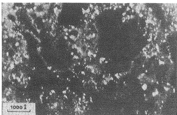
Figure 6. Agglomeration of chromium particles with matrix material viewed by TEM at 100 kV. The dark field shows metallic chromium particles as white spots. The dense black regions are holes produced by ion thinning.
