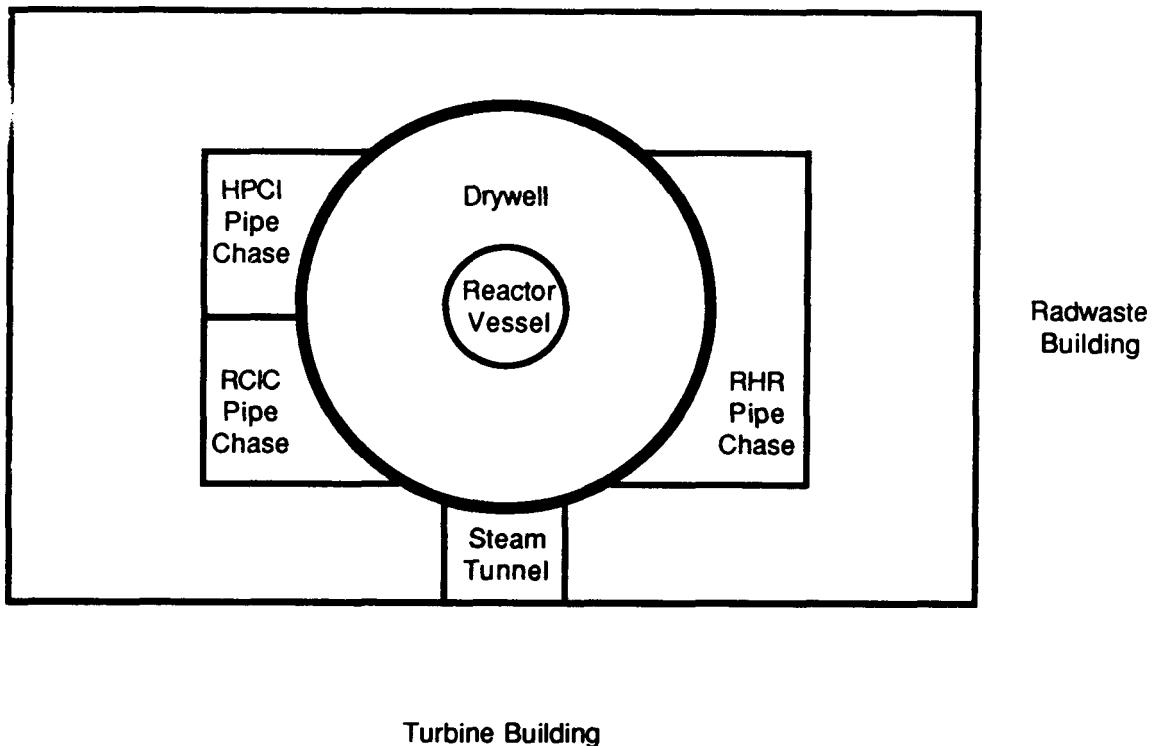
**Figure 6-4. Layout of Reactor Building at Grade Level.**
