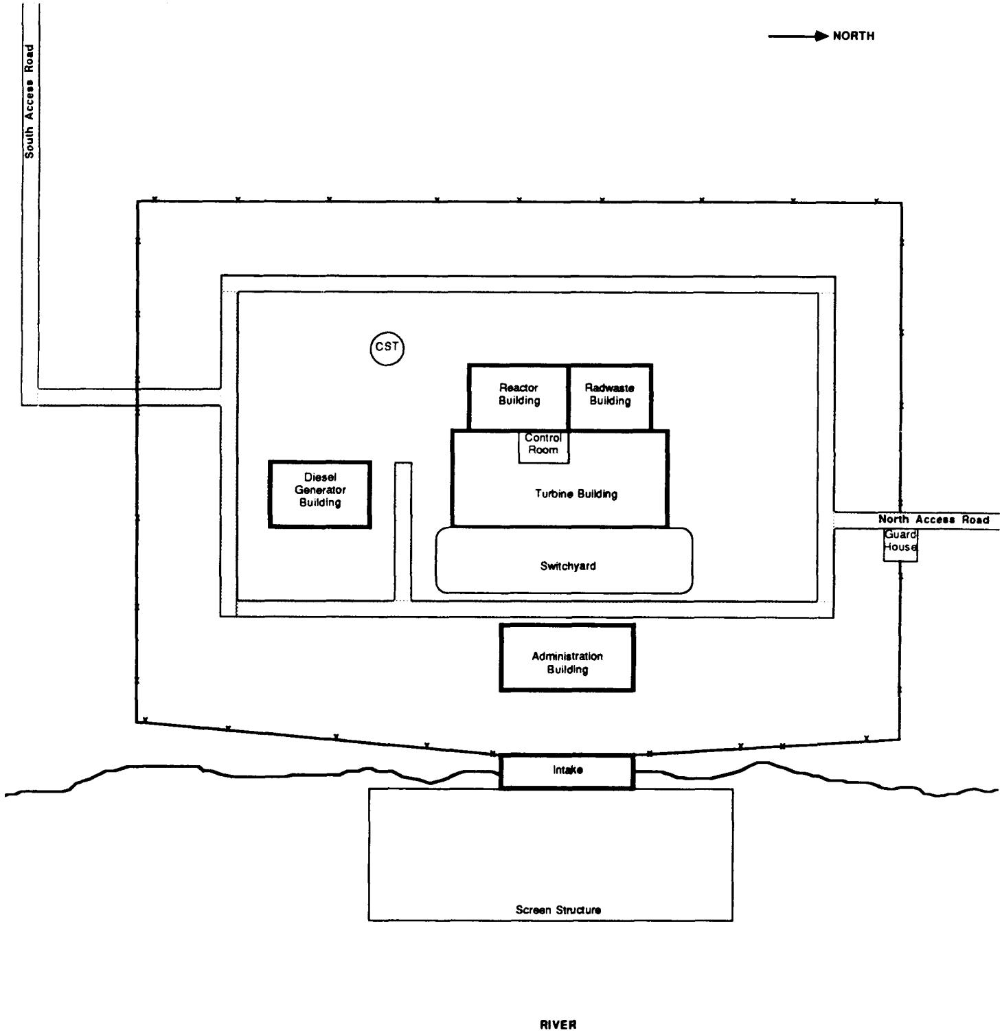
**Figure 6-1. Simplified Plot Plan of Sunshine BWR Plant**
