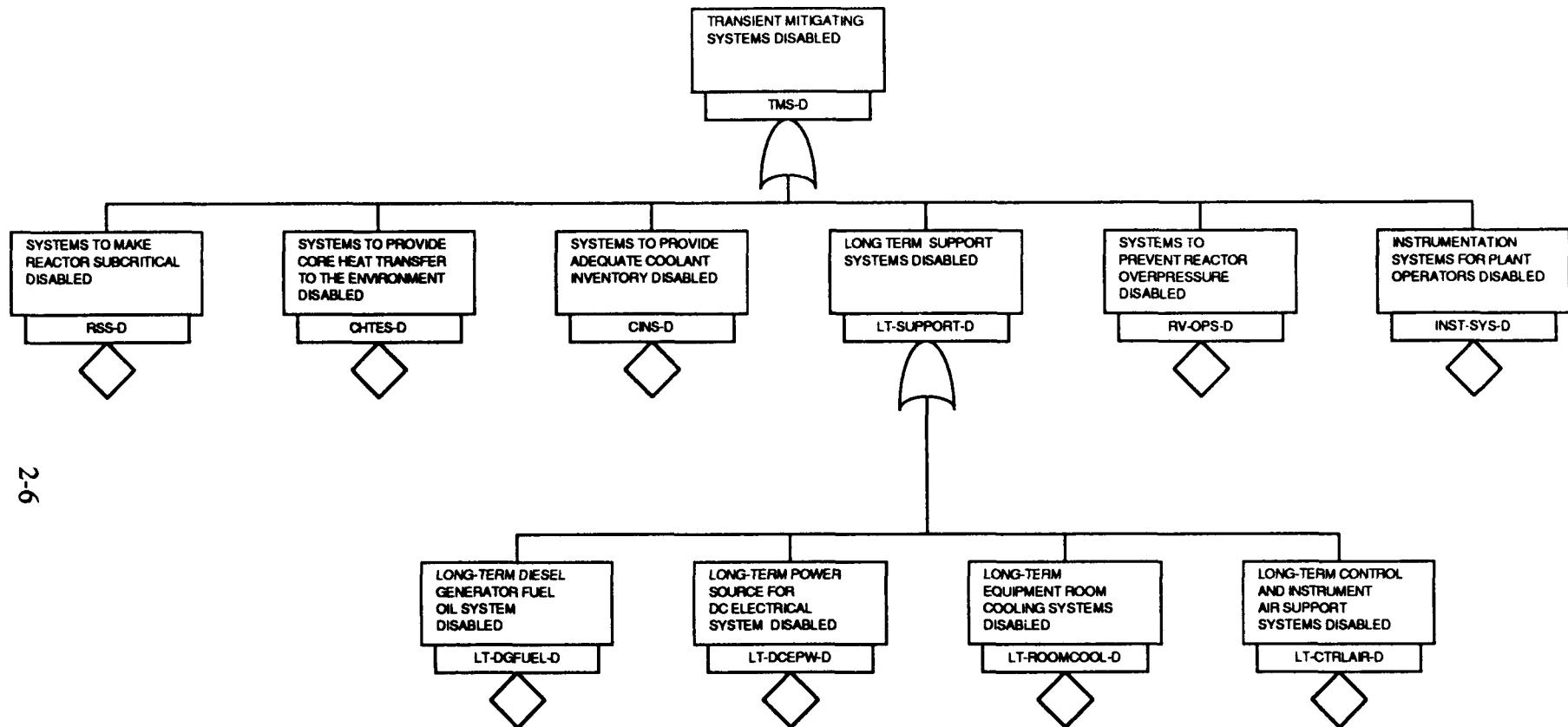
Figure 2-2. BWR Transient Mitigating System Fault Tree.
