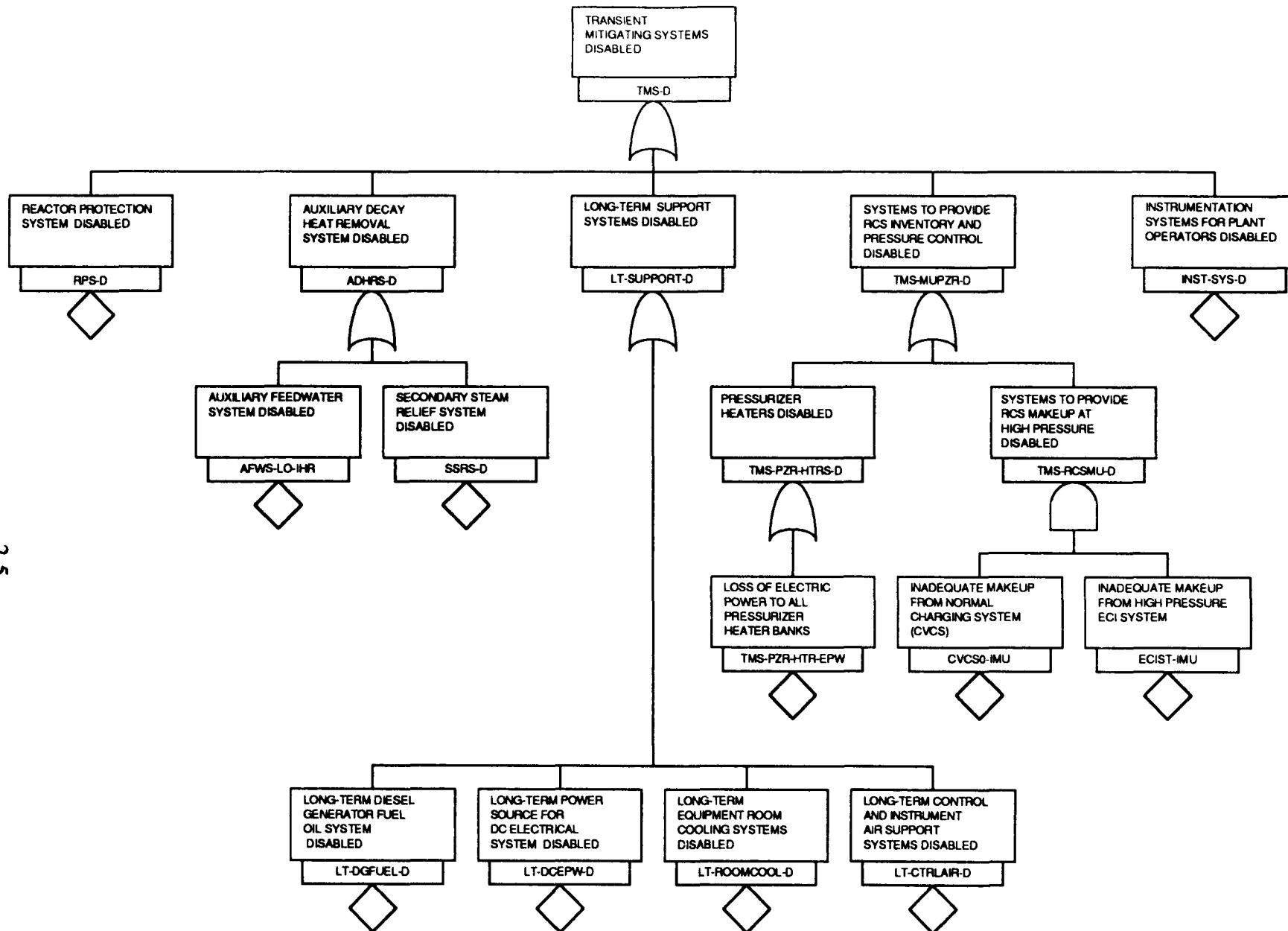
Figure 2-1. PWR Transient Mitigating System Fault Tree.
