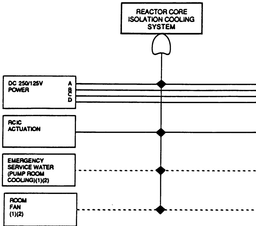
Dependency Diagram Is Shown Using Failure Logic.
