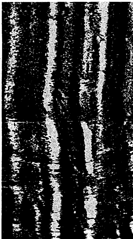
Figure 4. Image from 4500 to 4540 ft depth. The close-spaced discontinuous traces between about 4525 and 4530 ft are probably foliation.
