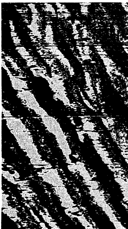
Figure 9. Image from 5000 to 5040 ft depth. The artifacts appear to be the same as for Figure 7. The obliquity may be due to the wellbore being rifled, the tool being badly off-centered, or failure of the magnetometer trigger.
