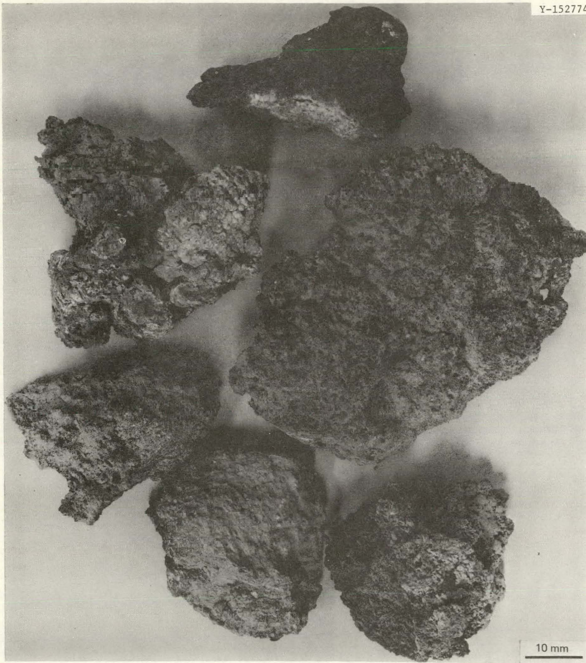
Fig. 3. Pieces of Degraded Brick.
