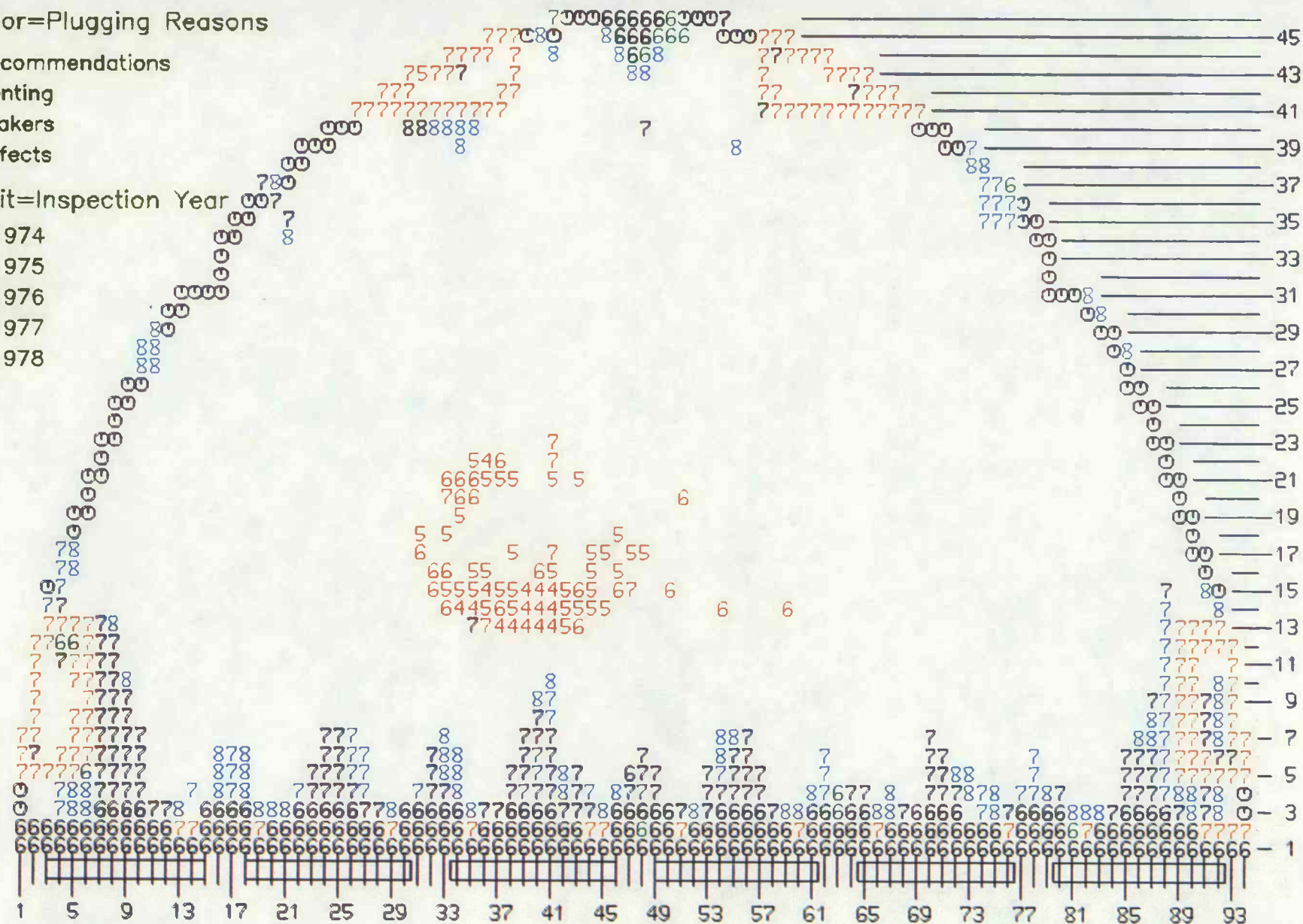
FIGURE 3. Tube Plugging Map of Surry 2A Steam Generator, Detailing Reasons for Plugging
