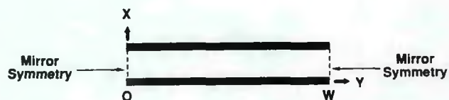
Figure 7. (a) The geometry a parallel-plate line.
