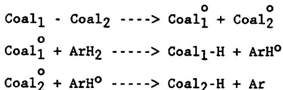
In this mechanism the  $\text{ArH}_2$  refers to a hydroaromatic moiety with two donable hydrogen atoms and Ar is an aromatic species. The TRC mechanism seems plausible when viewed in light of coal molecular structure, which is thought to be that of polycondensed aromatic clusters connected by linkages such as methylene, ether, and sulfide groups. The major question seems to be, are these linkages broken in a purely thermolytic unimolecular process, or by some other mechanism?
