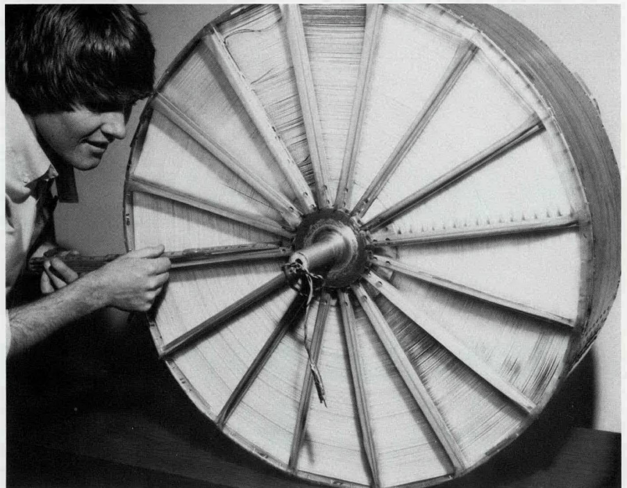
Experimental desiccant wheel for a dehumidifier cooling system.
