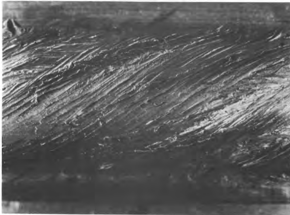
FIGURE 8. Groove of Unhardened D/d = 20 Sheave After 250,000 Bending Cycles
