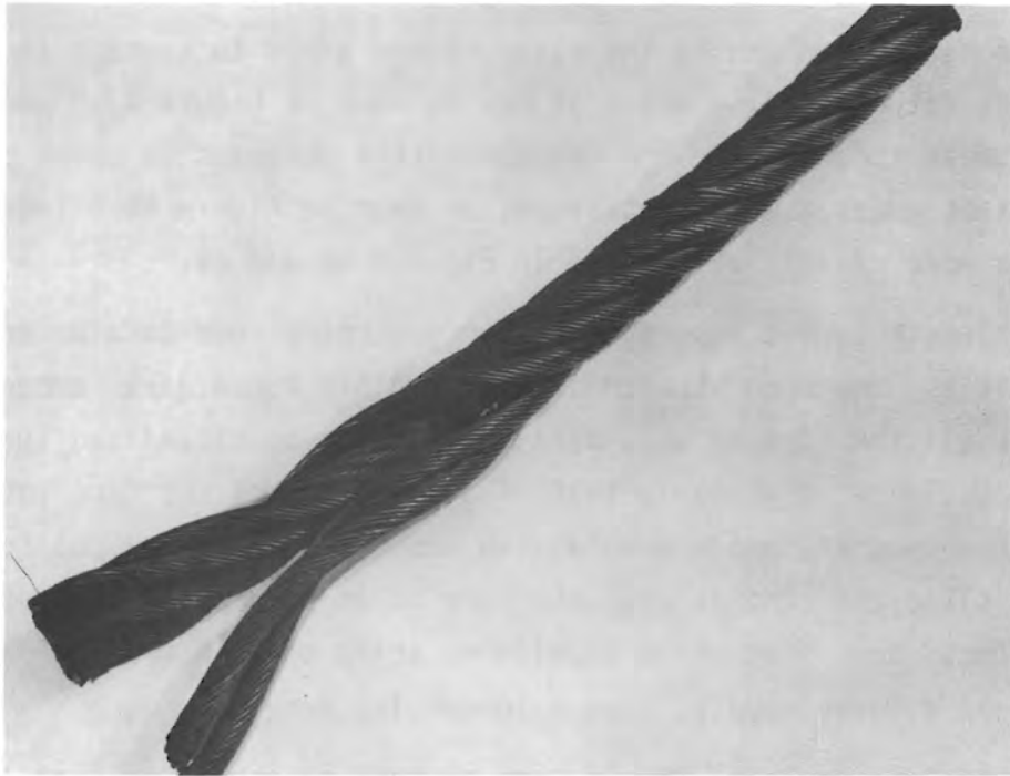
FIGURE 43. General View of IWRC Rope with Two Strands Twisted Out
