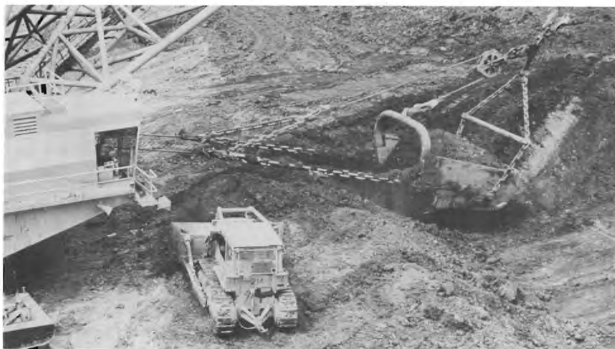
FIGURE 39. Bucket with Bale and Single Dump Rope System
