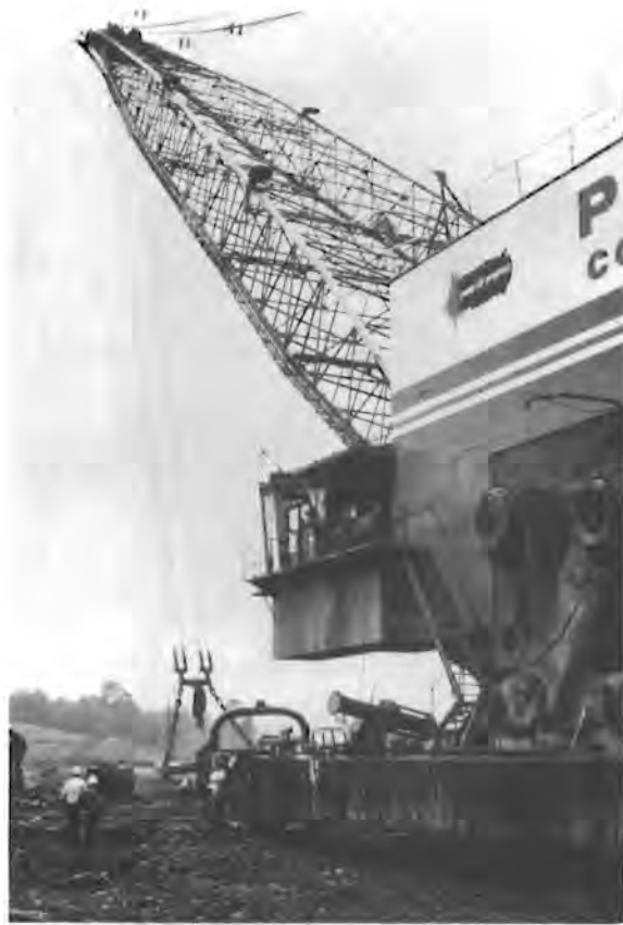
FIGURE 36. Four-Rope Hoisting System on Walking Dragline
