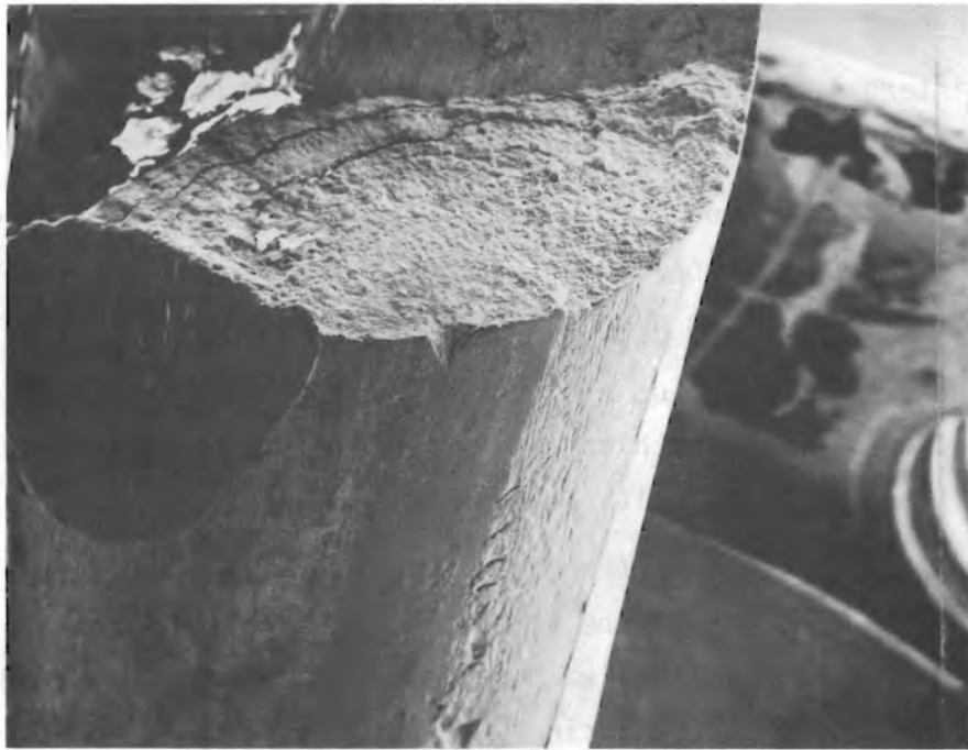
FIGURE 16. Fracture Surface of Wire Shown in Figure 15
