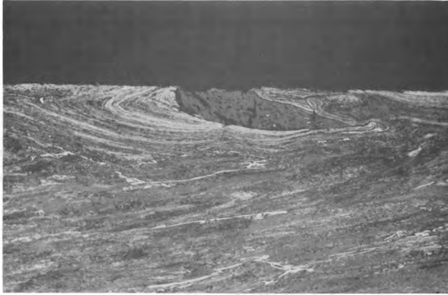
FIGURE 23. Section of Outer Wire from Rope Exhibiting Abrasive Wear
