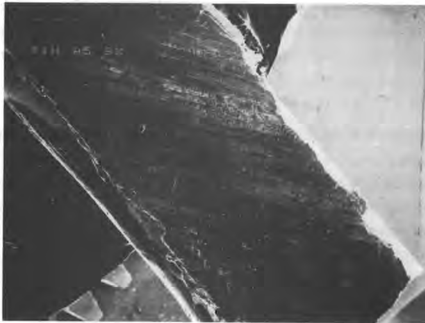
FIGURE 21. Wire Section Flattening and Surface Extrusion in Outer Wire Wear
