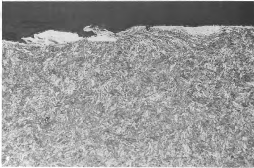
FIGURE 25. White Etching Layer on Worn Wire from Field Rope
