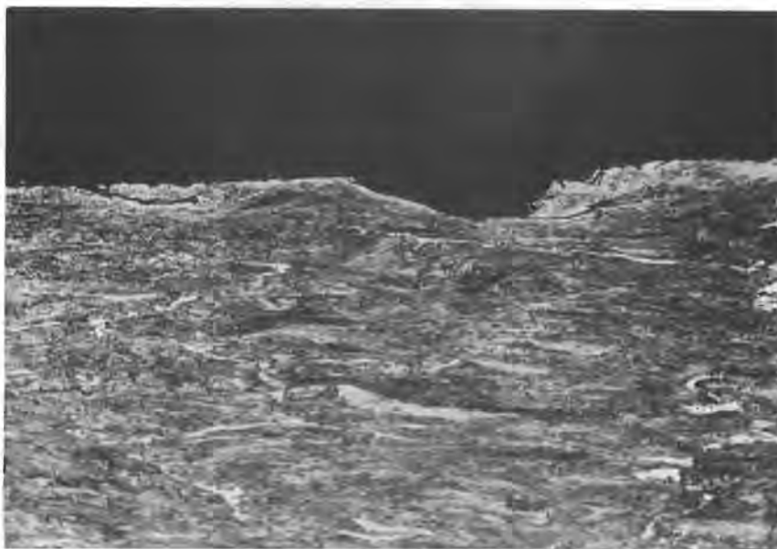
FIGURE 28. Delamination Wear in a Strand-to-Strand Notch
