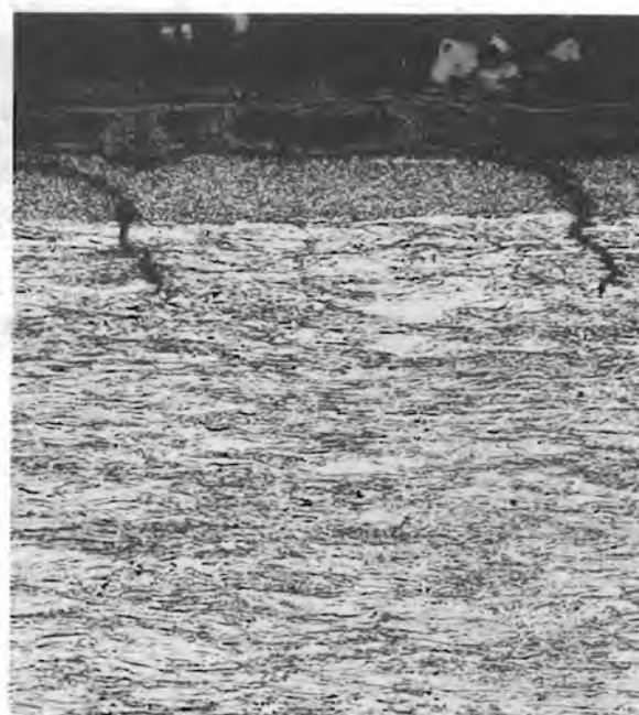
d. Longitudinal Wire Section Along Minor Contact Area (250X)
