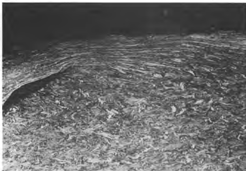
FIGURE 20. Deformation and Extrusion in the Notch-Forming Process
