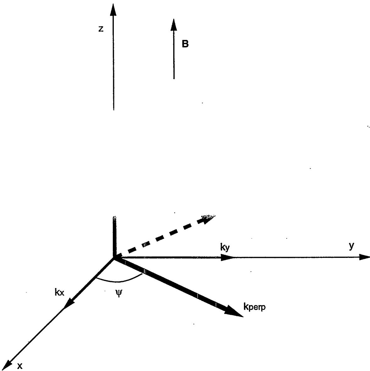
Figure 1: Local Cartesian coordinate system used to obtain the hot plasma dispersion relation. The magnetic field,  $\mathbf{B}$ , is assumed to lie along the  $z$ -axis perpendicular to the  $x,y$ -plane. The wave vector,  $\mathbf{k}$ , is represented by components parallel and perpendicular to the magnetic field.
