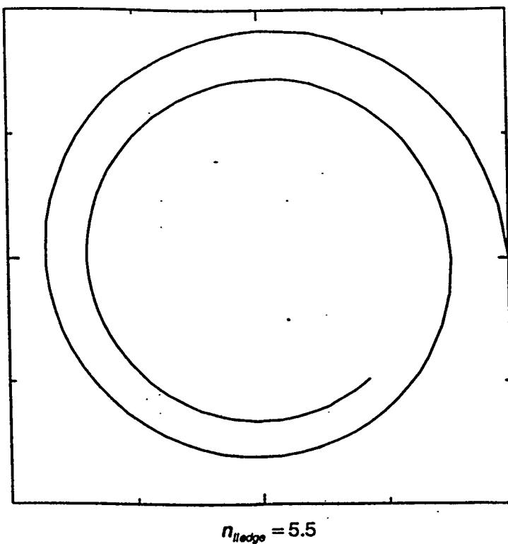
Figure 13: Ray trajectory in a constant toroidal angle plane for RFX where  $n_{\text{edge}} \approx 5.5$ . The ray is launched at the wall and makes slightly less than two poloidal transits before being completely absorbed by the plasma.
