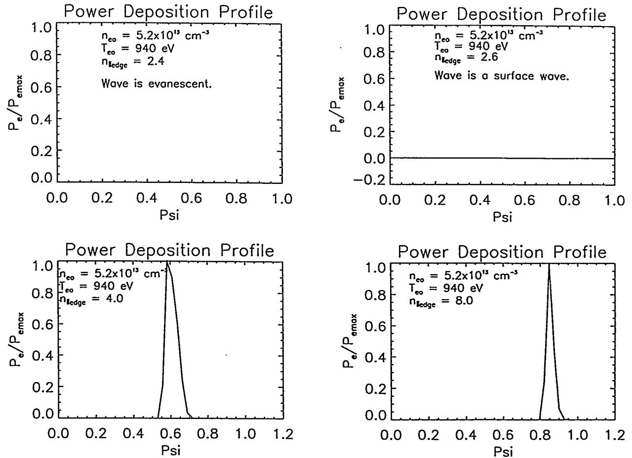
*Figure 16: Power deposition profiles for the cases discussed in Figure 15. Note that the electrons receive maximum power at c)  $\psi = 0.6$  for  $n_{lledge} = 4.0$  and d)  $\psi = 0.85$  for  $n_{lledge} = 8.0$ .*
