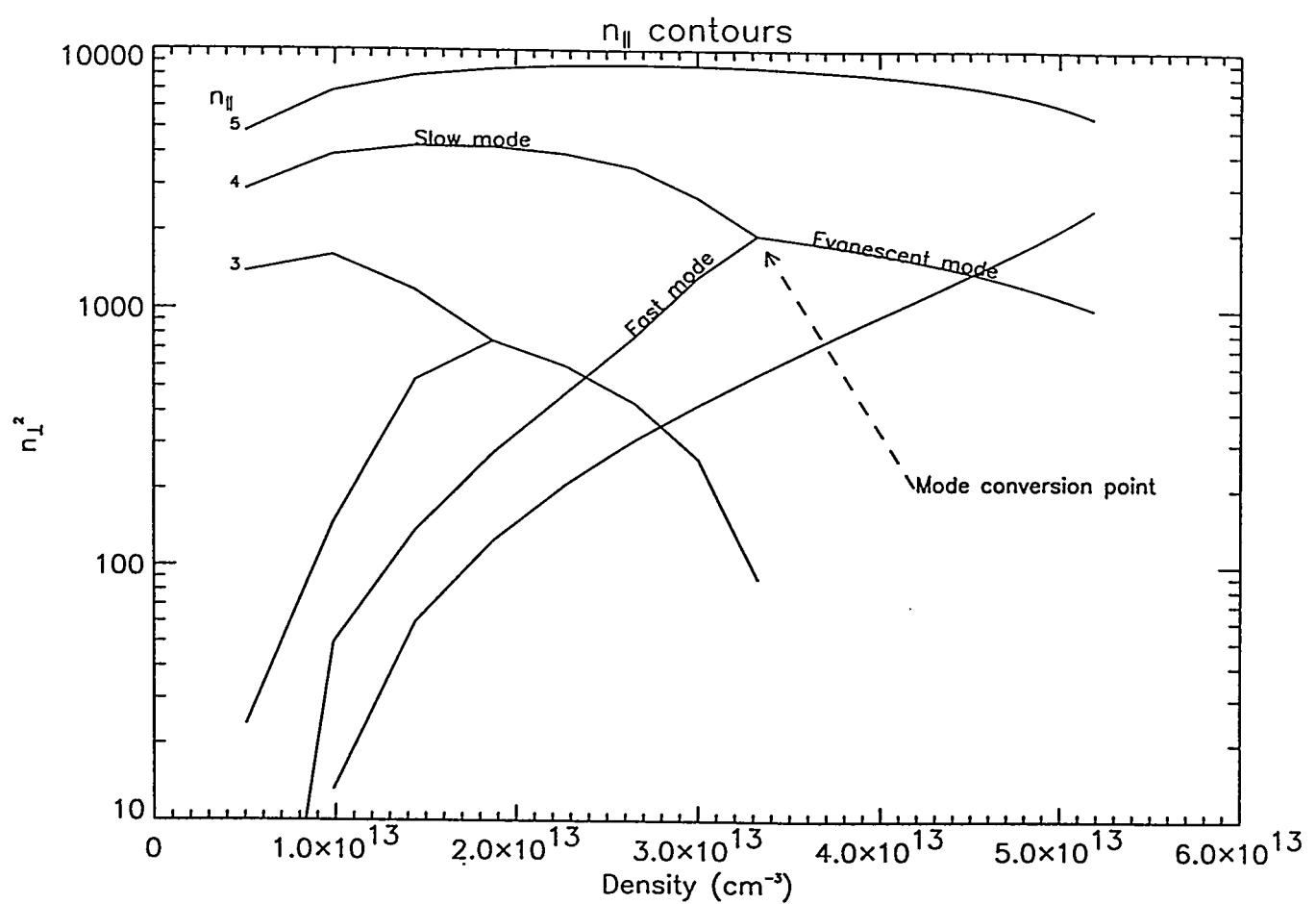
*Figure 10: Plots of values of  $n_{\perp}^2$  for the slow and fast wave as density increases for selected values of  $n_{\parallel}$  in RFX. The extra path at the mode conversion point is an evanescent mode inside the cutoff.*
