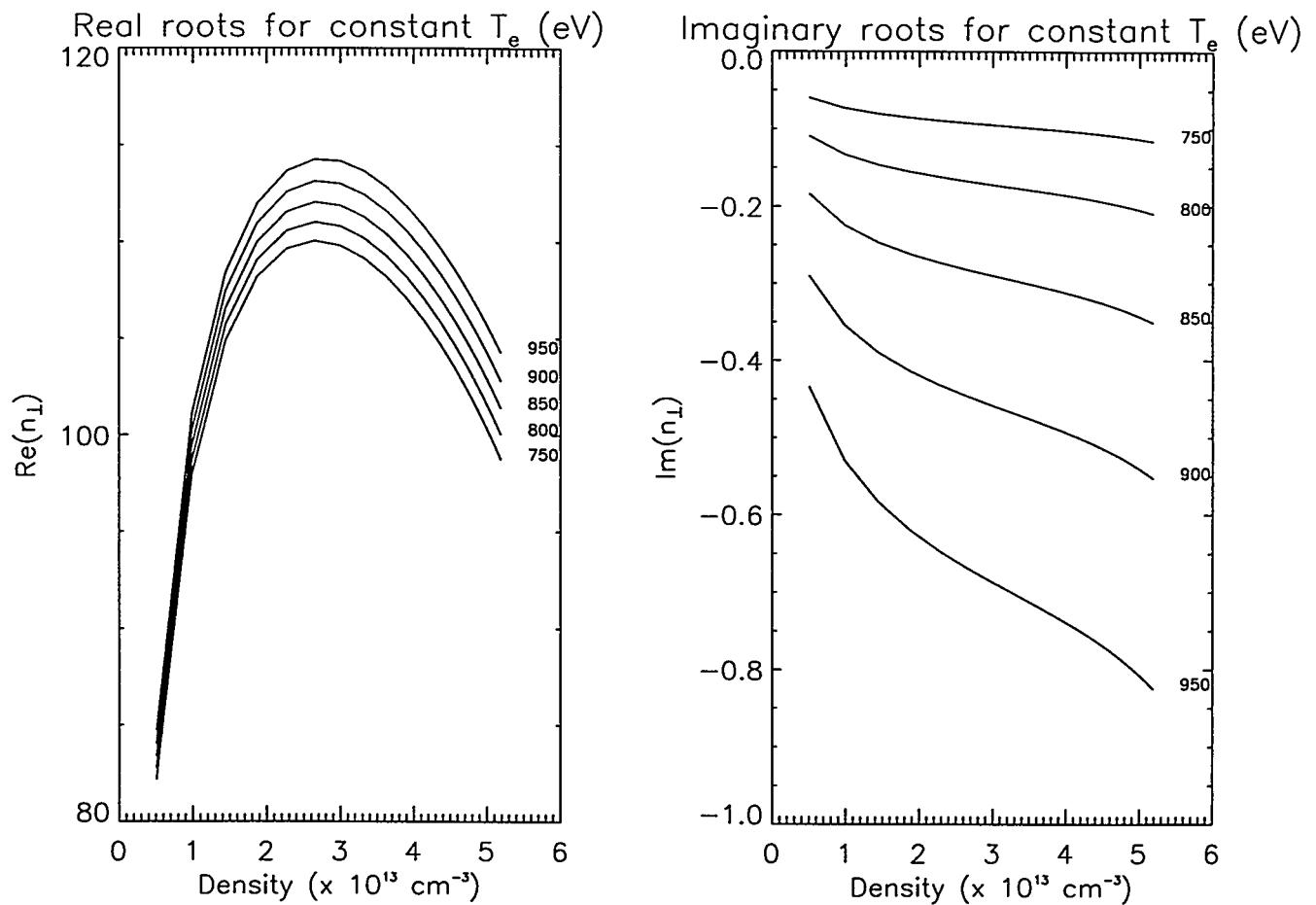
*Figure 5: Behavior of the roots of the hot plasma dispersion relation for constant values of temperature. The real part of the function shows little dependence upon temperature. However, the imaginary part shows strong wave damping as temperature increases.*
