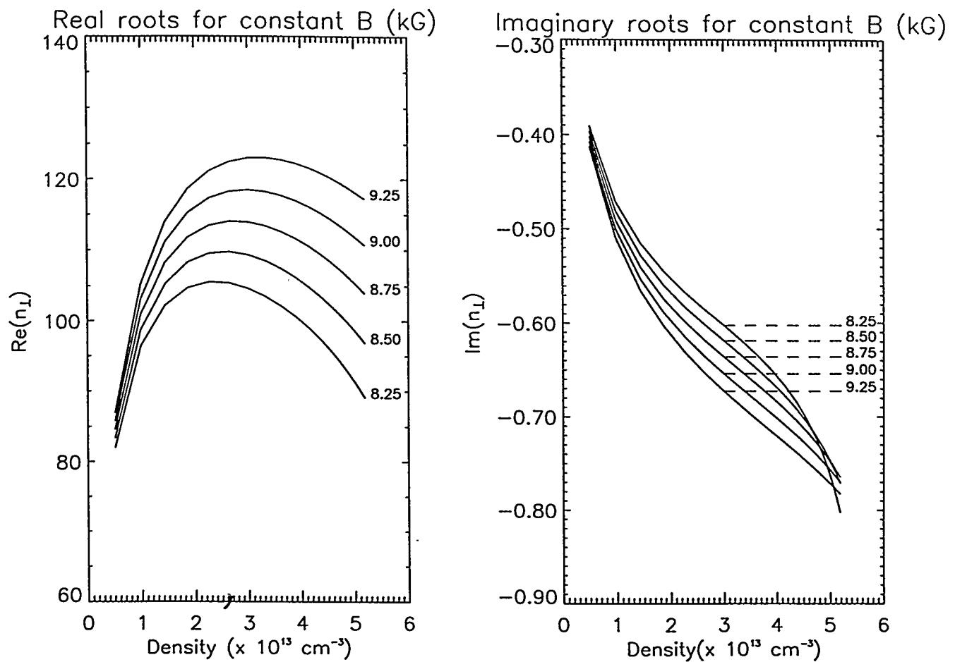
*Figure 6: Behavior of the roots of the hot plasma dispersion relation for different values of magnetic field strength. The curves show a monotonically increasing dependence of the roots on  $|B|$ .*
