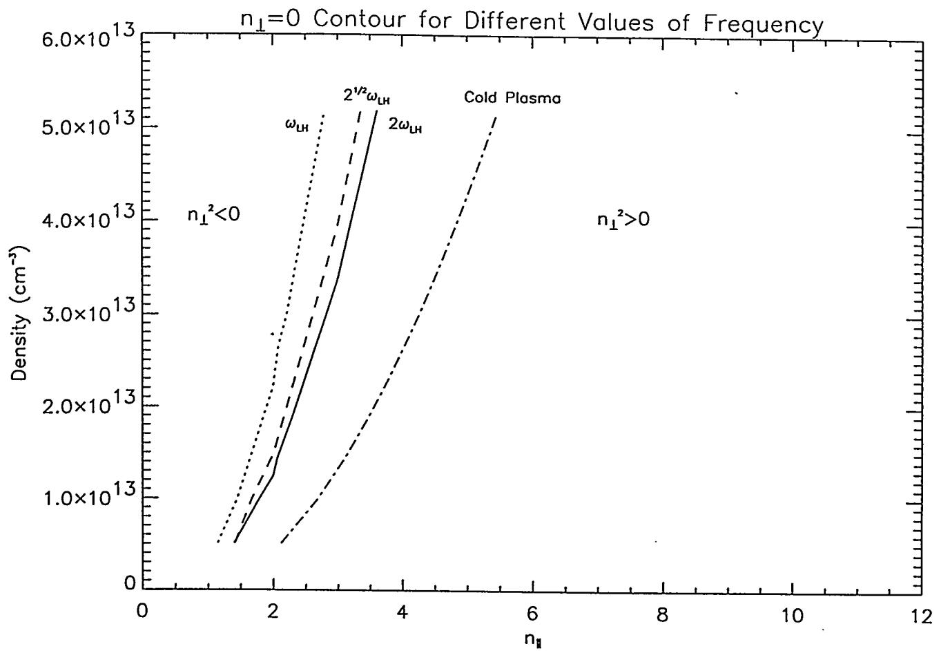
Figure 8: Contour plot of  $n_{\perp}^2 = 0$  for RFX at  $I/N = 6 \times 10^{-14} \text{ A}\cdot\text{m}$  and  $T \rightarrow 0 \text{ eV}$  for different values of wave frequency. Here, dotted lines correspond to  $\omega \approx \omega_{LH}$ , dashed lines correspond to  $\omega \approx \sqrt{2}\omega_{LH}$ , and solid lines correspond to  $\omega \approx 2\omega_{LH}$ . The cold plasma cutoff is also present (dot-dash lines).
