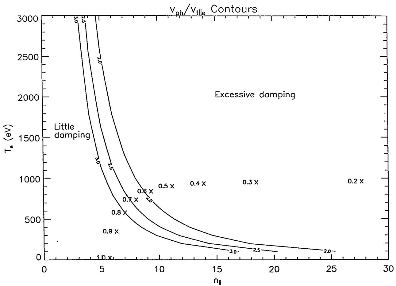
Figure 11: Contours of  $v_{ph}/v_{tle}$  over parallel index of refraction and temperature. Uchimoto predicts that optimal Landau damping occurs where  $v_{ph}/v_{tle} \approx 2.5$ . The path of the ray is marked by 'x' and labeled with the corresponding value of  $r/a$ . Here, the ray is located for ideal Landau damping in the region  $r/a \approx 0.7$ .
