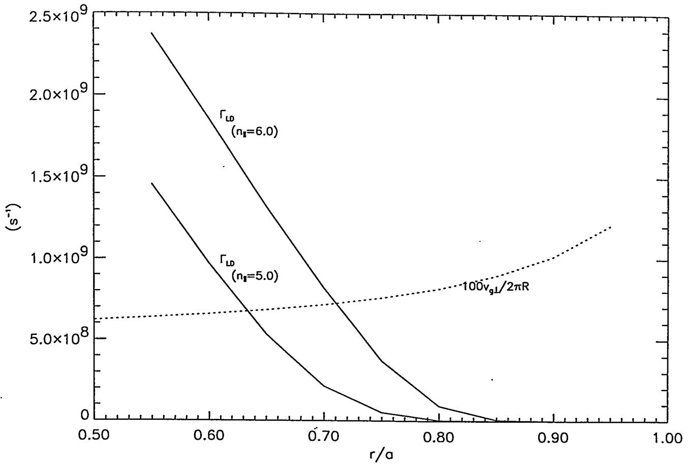
Figure 12: Landau damping rate (solid) versus  $100v_{g1}/2\pi R$  (dotted) as a function of  $r/a$  for the cases of  $n_{\parallel\text{edge}} = 5.0$  and  $n_{\parallel\text{edge}} = 6.0$ . The point of intersection of the two curves marks the region of ideal Landau damping. Since the two points fall on either side of  $r/a = 0.7$ , we estimate that the ideal  $n_{\parallel\text{edge}} = 5.5$ .
