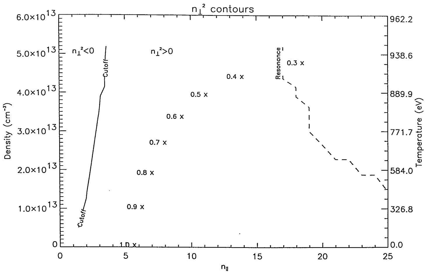
**Figure 9:** Contour plot of  $n_{\perp}^2 = 0$ . The path of the wave through the plasma has been marked by 'x' and labeled with the corresponding  $r/a$  value. The dashed curve shows the region of the resonance between the wave parallel phase velocity and the electron parallel thermal velocity.
