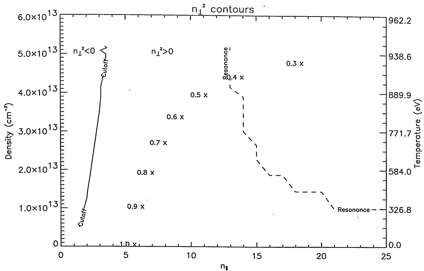
Figure 18: As in Figure 9, but for an RFX plasma with 10% hot electrons. Note that the thermal resonance has shifted to lower  $n_{\parallel}$ .
