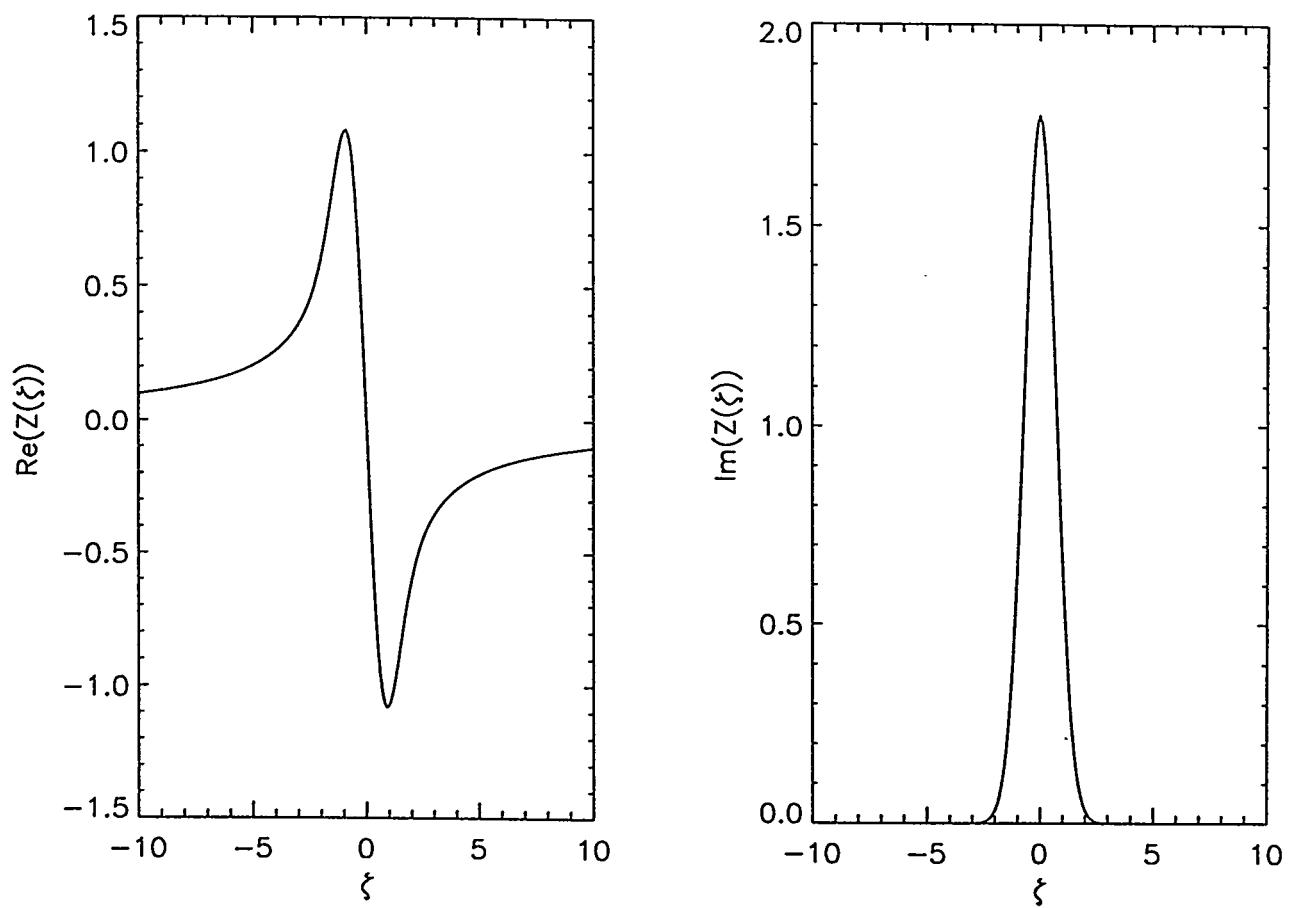
*Figure 2: Real and imaginary values of the plasma dispersion function as determined by the function ZFUNC.*
