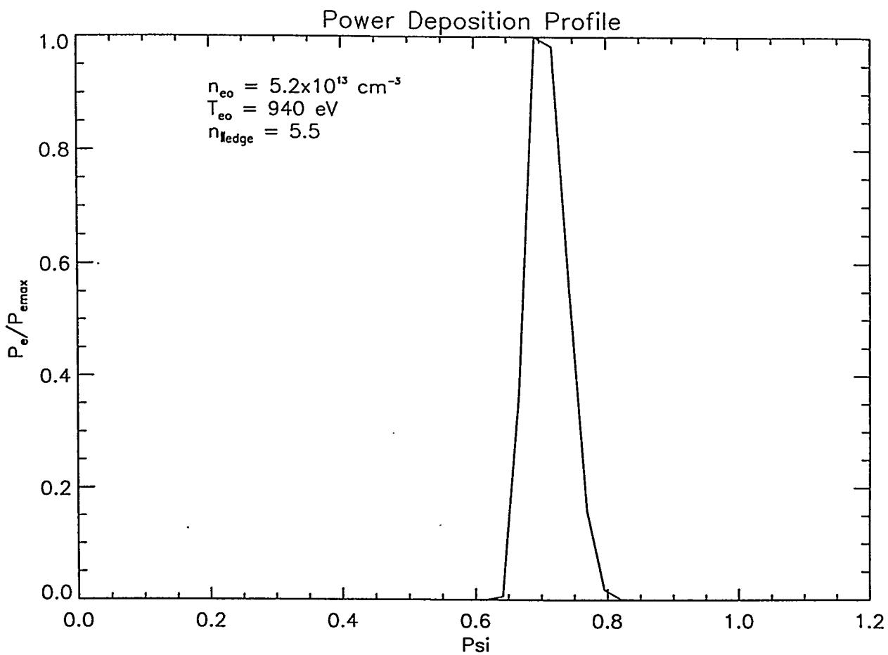
*Figure 14: Power deposition profile for the lower hybrid wave launched into RFX with  $n_{edge} = 5.5$ . The spike located at  $\psi \approx 0.7$  ( $\psi$  is a flux surface coordinate analogous to  $r/a$ ) is indicative of a relatively large amount of power to the electrons at this point and, therefore, of current driven in this region. Power delivered to the ions was negligible.*
