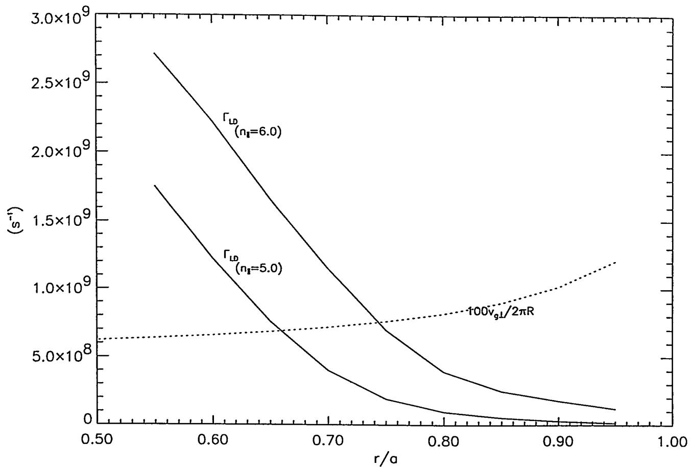
*Figure 20: As in Figure 4 but for an RFX plasma with 10% fast electrons. The ideal damping points for each figure have shifted toward the edge of the plasma. To maintain optimal damping, this corresponds to a 6% increase in the wave's phase velocity at the edge of the plasma.*
