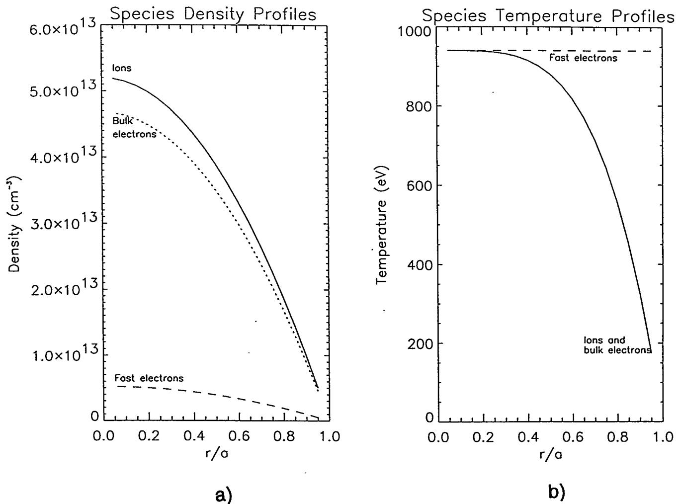
Figure 17: a) Assumed density and b) temperature profiles for RFX with a fast electron species present.
