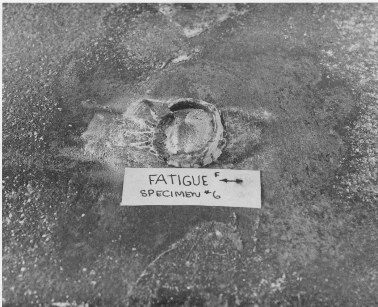
Fig. 22. Detail of failed stud, liner side - specimen No. 6 ( \pm 0.025 -in. controlled displacement)
