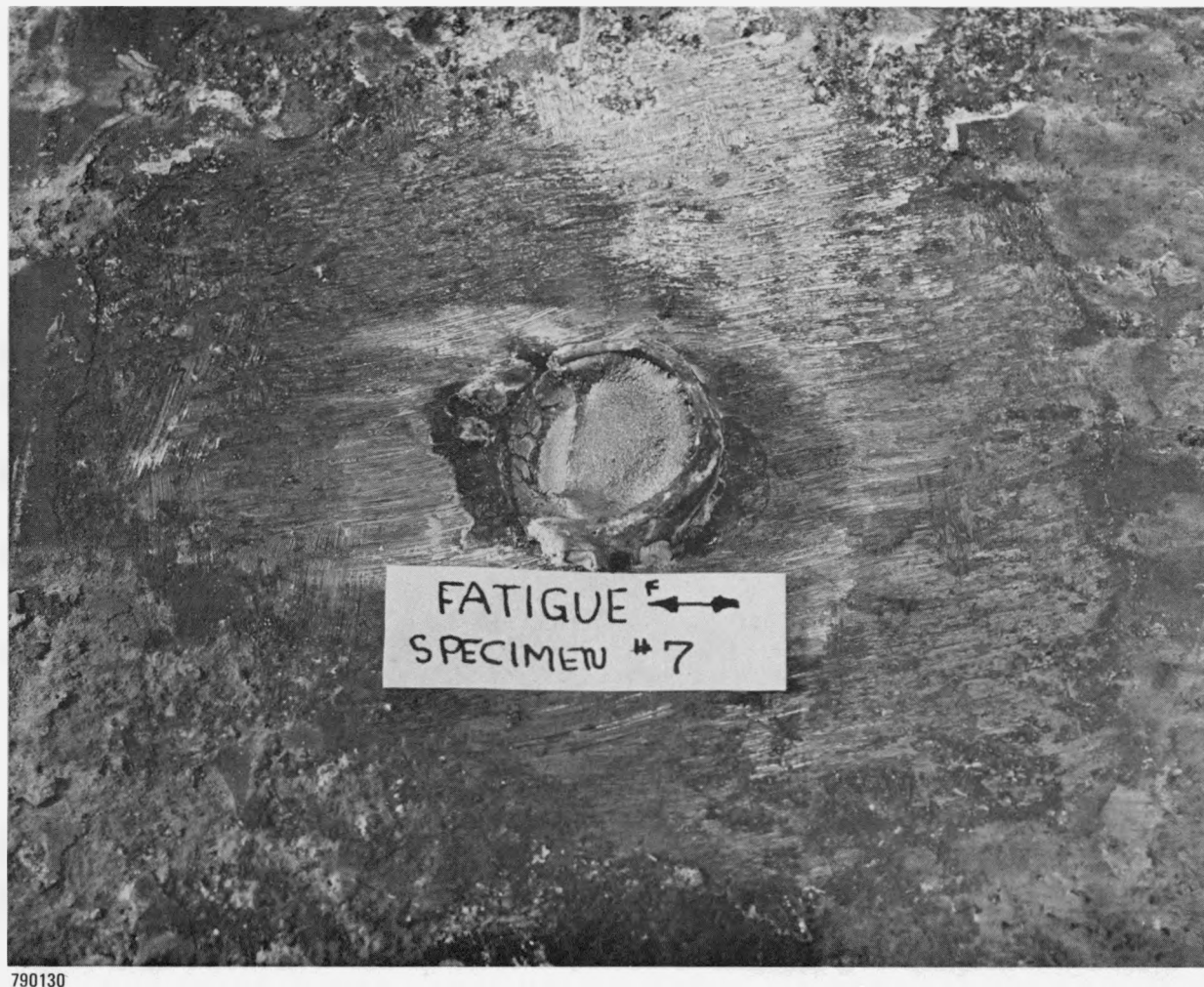
Fig. 19. Detail of failed stud, liner side - specimen No. 7 ( \pm 0.018 -in. controlled displacement)
