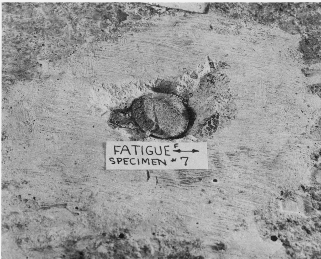
Fig. 20. Detail of failed stud, concrete side - specimen No. 7 ( \pm 0.018 -in. controlled displacement)
