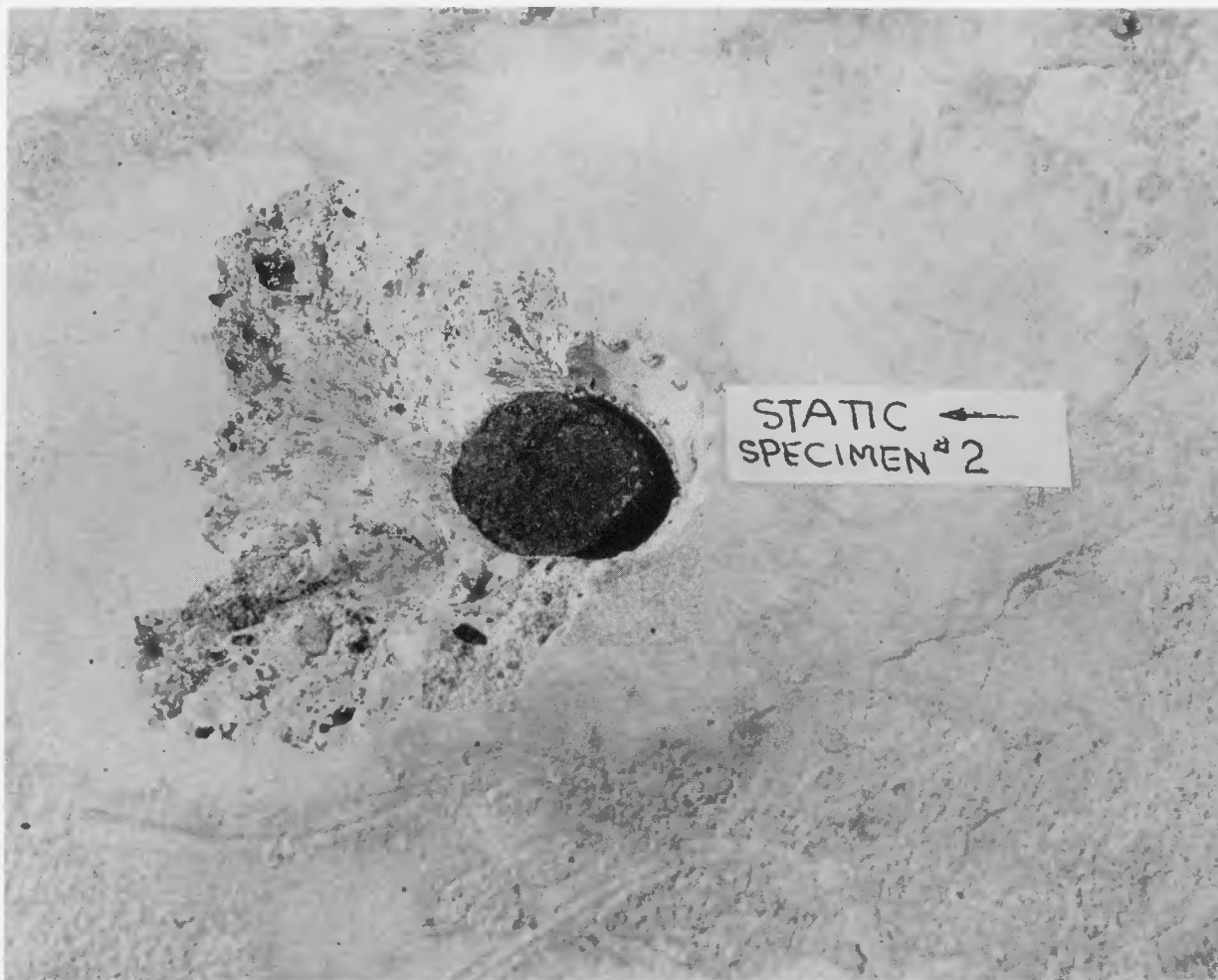
Fig. 6. Detail of stud, concrete side - monotonic test on specimen No. 2
