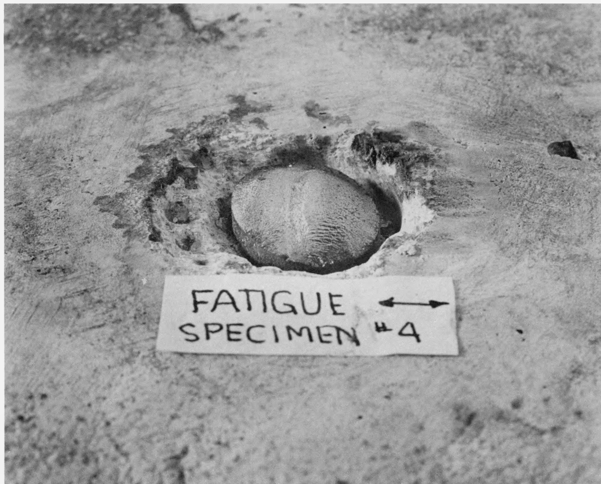
Fig. 17. Detail of failed stud, concrete side - specimen No. 4 ( \pm 0.012 -in. controlled displacement)
