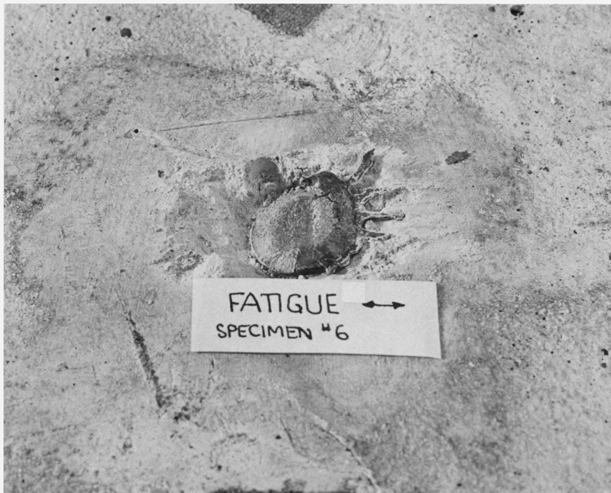
Fig. 23. Detail of failed stud, concrete side - specimen No. 6 ( \pm 0.025 -in. controlled displacement)
