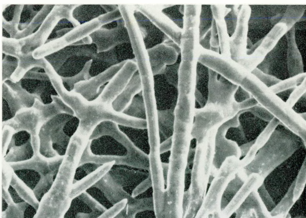
Fig. 3. Electron micrograph of the new stainless steel filter medium.
