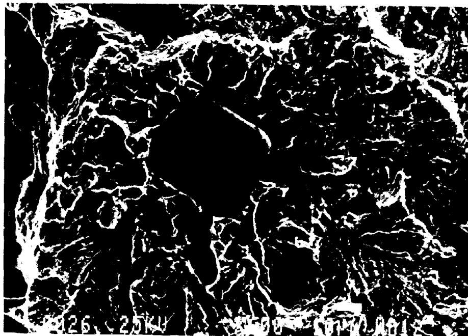
Fig. 30 SEM micrographs of a manganese sulfide inclusion completely surrounded by brittle-like fracture. Features such as this, which must have occurred ahead of the location of the crack tip, suggest that hydrogen might have assisted the fracture. Specimen is FOK-32, \Delta K = 48 \text{ MPa}\sqrt{\text{m}} . Fig. 30b is an enlargement of Fig. 30a.
