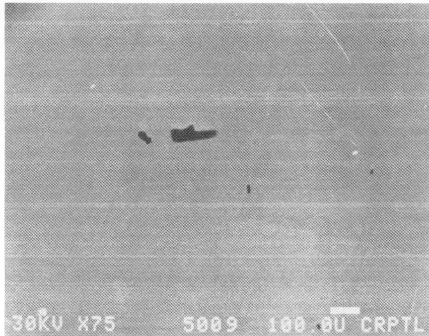
Figure 4-6. EBIC Image Of A PV Device Showing The Effect Of Surface Damage
