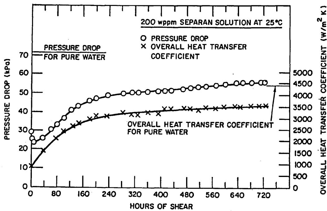
Figure 1. Pressure Drop and Overall Heat Transfer Coefficient as a Function of Circulation Time for 200 wppm Separan Solution at 25°C.
