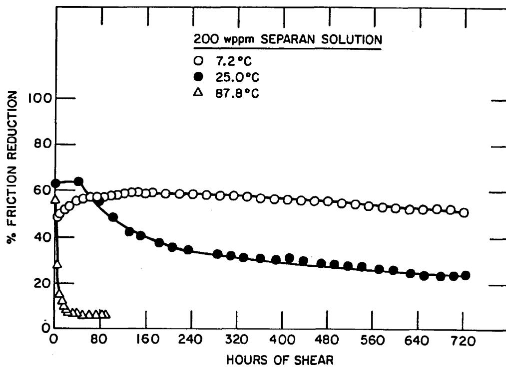
Figure 4. The Effect of Temperature on Percent Friction Reduction as a Function of Circulation Time for 200-wppm Separan Solution.
