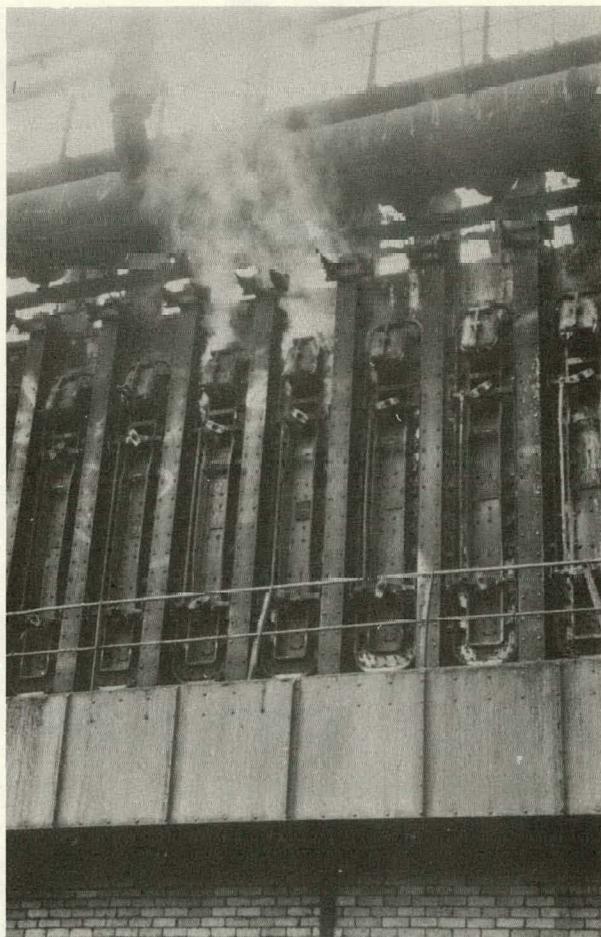
Fig. 6. Leaks from coke oven doors during operation.
