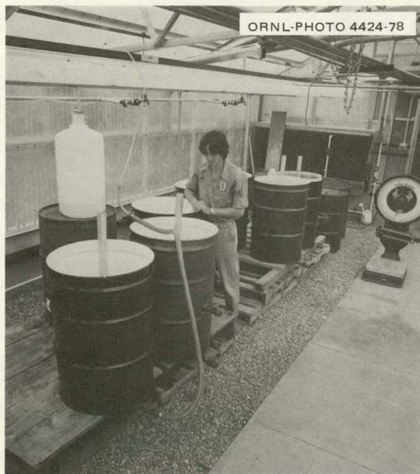
Fig. 4. Large ash/soil leaching columns.
