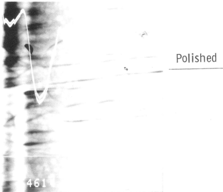
Figure 9. EBIC scan through the twin planes located on the polished web surface of crystal R461-4. This scan was taken 700 \mu\text{m} away from the bottom edge ( I_b = 270 \text{ pA} ).
