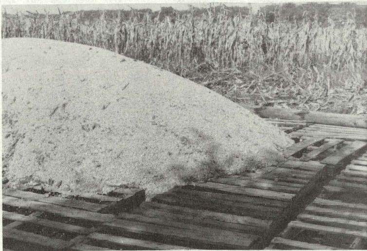
Pallets covered with plastic netting support the grain and provide an air duct to exhaust air that has been forced down through the grain.
