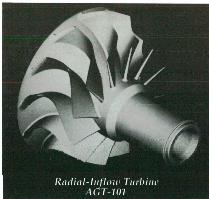
Figure 2. Radial and Axial Ceramic Turbine Rotors Designed for 2500°F Operation.
