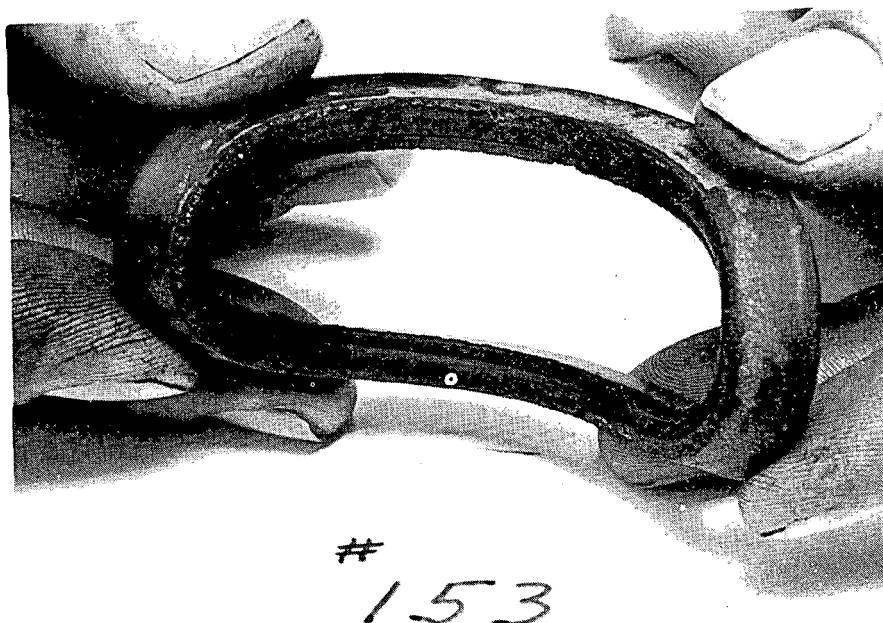
Figure 32. Peroxide-cured Viton run 53 hours in abrasives at 200°C.
