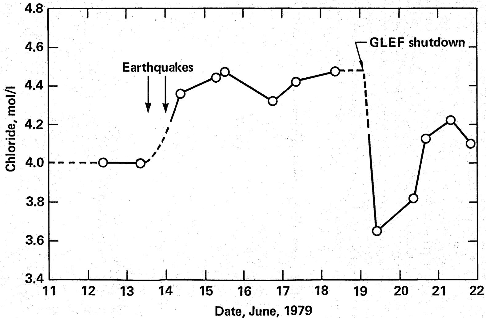
As can be seen in Figure 2, when the GLEF ceased operation on June 19, 1979, the salinity of the brine -- flowing at the reduced rate at the wellhead -- dropped precipitously. The new level (3.5-3.8 Mo/l chloride) was typical<sup>3,4,6</sup> of that observed when we were the sole user of the well, but then the brine salinity rose again to a level that may be the new equilibrium value. Our experiments were terminated on June 22nd.
