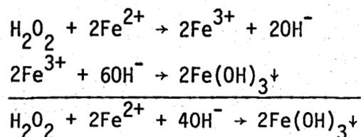
A "multiplication" factor thus could be created in which one mole of  $\text{H}_2\text{O}_2$  would result in the consumption of four moles of hydroxide ion. On a strictly per-pound basis, this would be more economical than using HCl.
