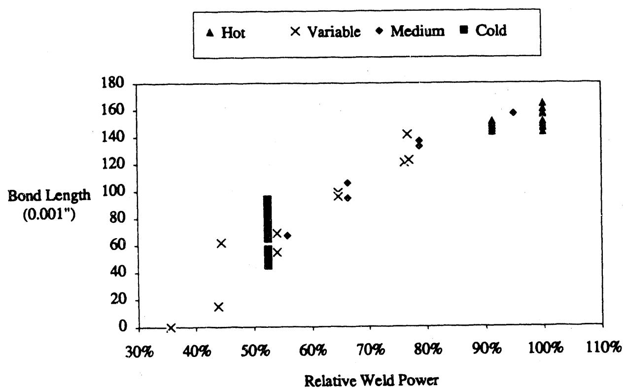
Figure 2. Pinch weld bond length versus relative weld power. Same welds as Fig. 1.
