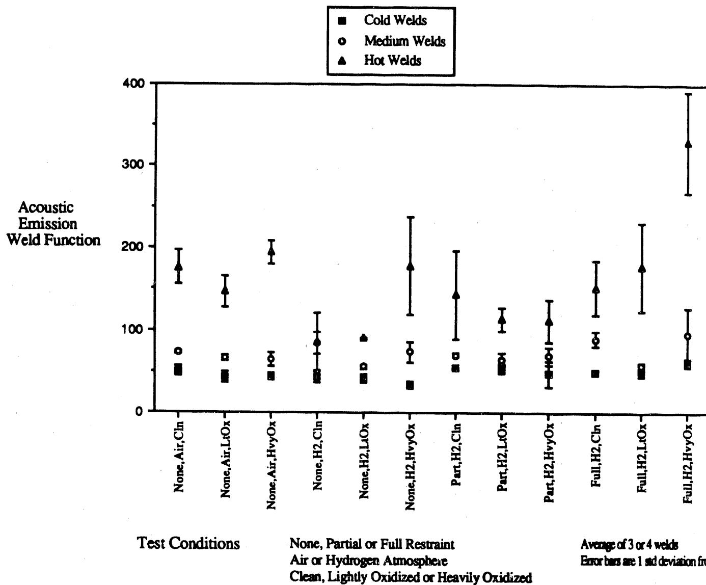
Figure 3. Acoustic emission weld function for previous study, for welds made at various conditions of restraint, atmosphere, and degree of oxidation as shown. Acoustic emission weld function is energy counts for a weld divided by weld power, this is roughly equivalent to the ringdown counts used in Fig. 1. Weld power levels Hot, Medium and Cold in this figure do not necessarily correspond to those of Figs. 1 and 2.
