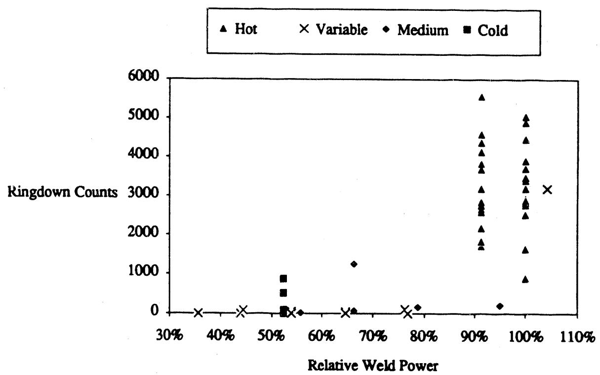
Figure 1. Acoustic emission ringdown counts versus relative weld input power. Experiments performed in four series, labeled "Hot", "Variable", "Medium", and "Cold" as shown.
