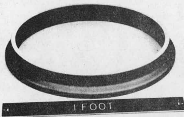
Fig. 17 12" diameter SiC insulating ring
