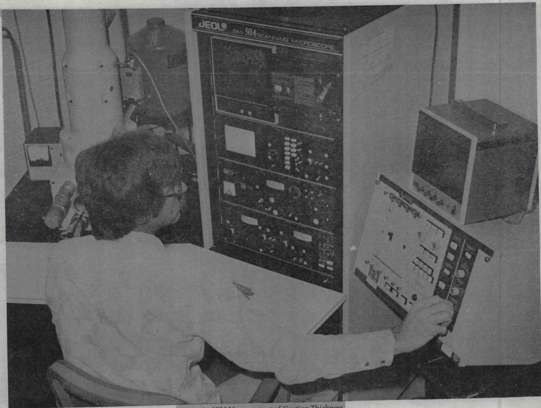
Figure 5. SEM Measurement of Coating Thickness
