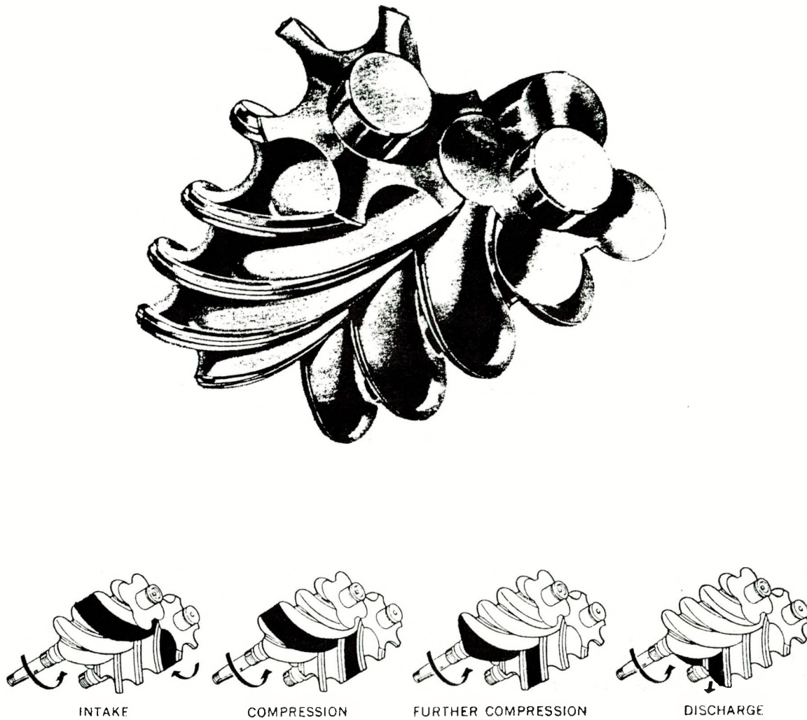
Figure 5.10 Screw Compressor Operation
