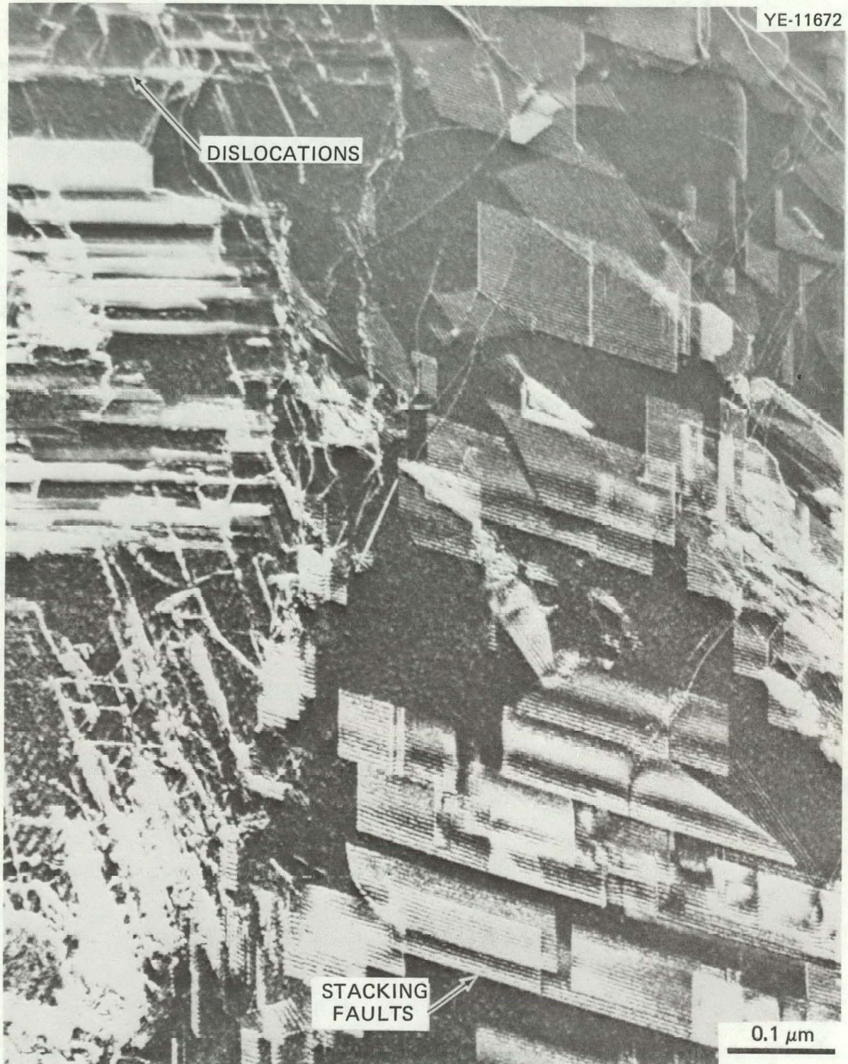
Fig. 7. Defects in SC472, Weak-Beam Dark-Field Image.
