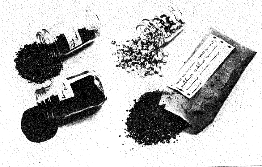
Figure 15. Examples of alloying agents added to crucible and/or mold.
