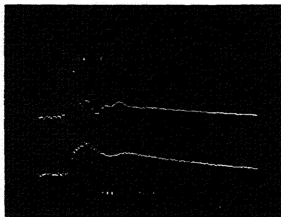
Figure 10 Voltage and current waveforms during a cable test; 15 kV cable, 4.6 m long, terminated in 60 ohms; 500 ns/div, 91.6 kV/div, 158 kA/div, 341 kV peak, .773 kA peak.
