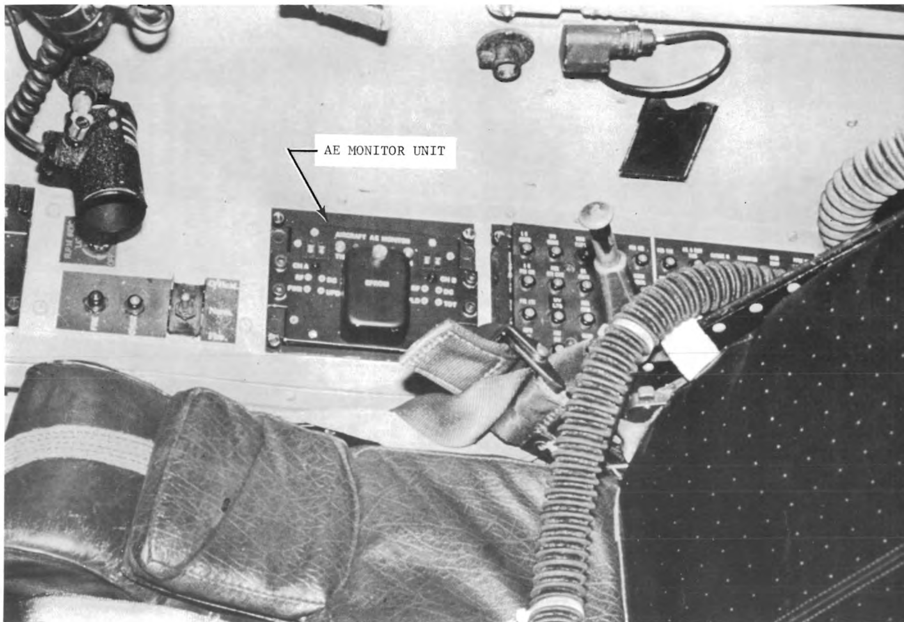
Figure 18. AE Monitor Unit Installed in Macchi Aircraft A7-021.
